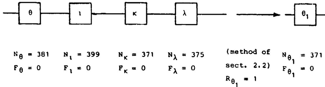
\*This warhead component is repeated in other subsystems but, since it is being treated as having essentially an infinite number of trials, it cannot affect calculation of the equivalent N and so it can be treated as independent, affecting only the calculation of R.
