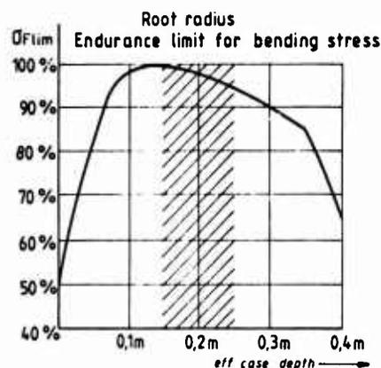
Namely : 1. On the flanks a minimum effective case depth larger than the "depth of maximum shear stress" is asked but no maximum because this maximum does not decrease the strength against Hertzian pressure.
