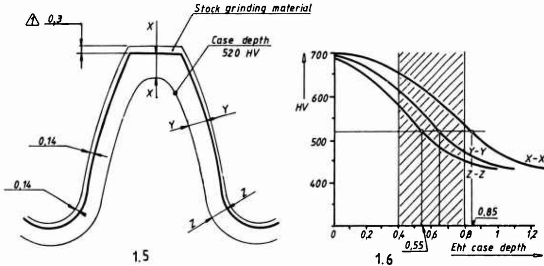
A second corrective action is applied to the following fabrication lot. Besides enlarging the outside diameter we also modify the tooth thickness at the tip. We realize this by using a hob with a special basic profile.
