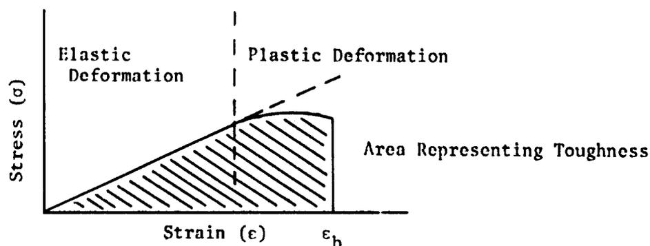
Fig. 1. Typical Stress/Strain Curve
