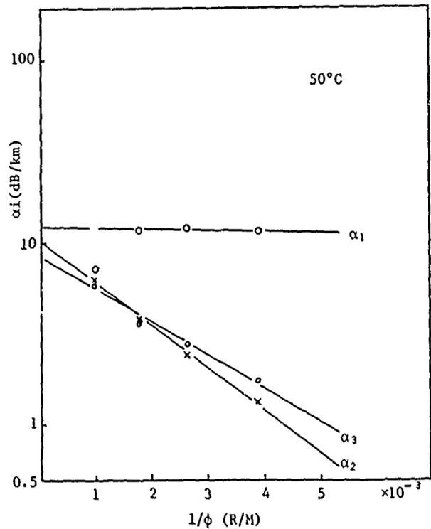
Fig. 13 Dose Rate Dependence of  $\alpha_i$  ( $50^\circ\text{C}$ )
