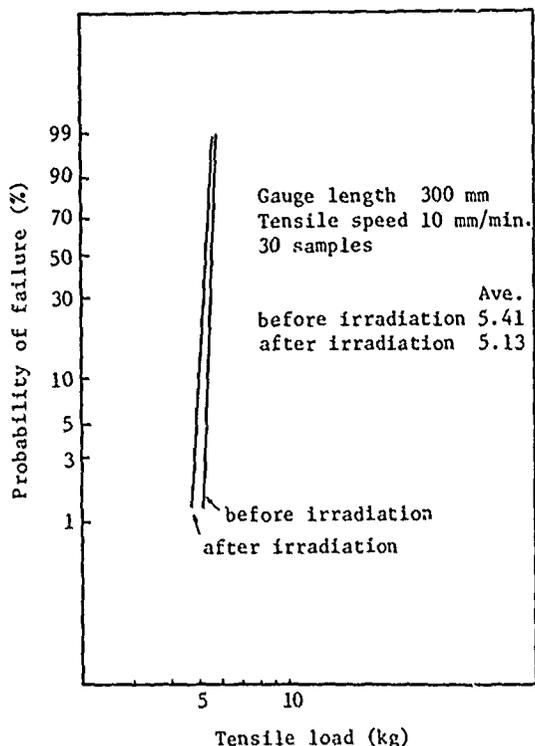
Fig. 22 Tensile Strength before and after Irradiation
