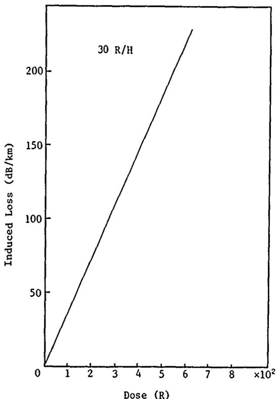
Fig. 5 Radiation-induced Loss (P Doped Core SI Type)
