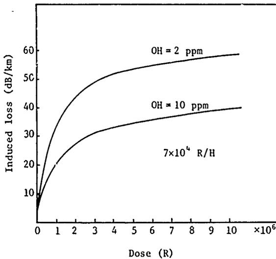
Fig. 7 Radiation-induced Loss (Pure Silica Core Fiber)
