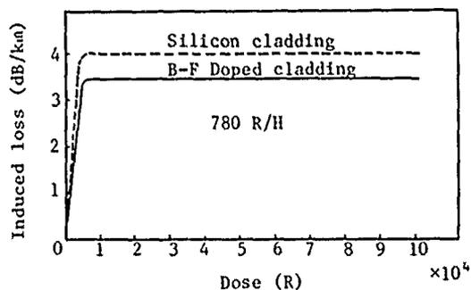
Fig. 6 Radiation-induced Loss (Pure Silica Core Fiber)
