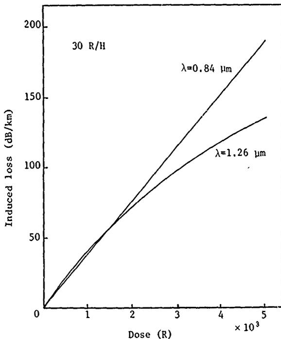
Fig. 2 Radiation-induced Loss (Ge-P Doped Core GI Type)
