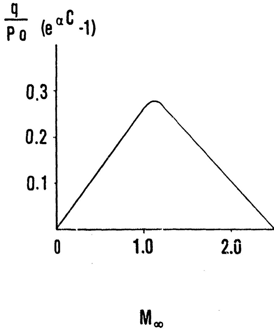
Figure 6. Relative Intensity of Disturbances for Different Mach Numbers
