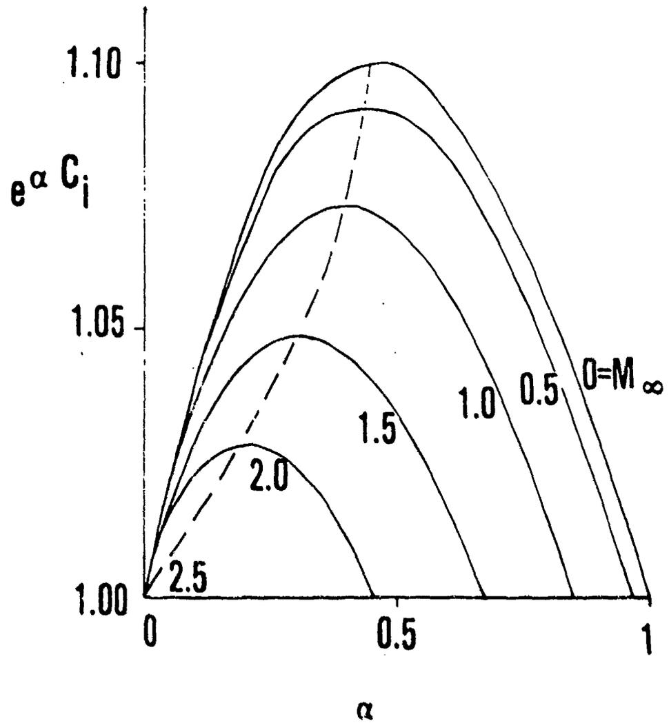
Figure 4. Amplification Factor v.s. Wave Number for Different Mach Number (Ref. 12)
