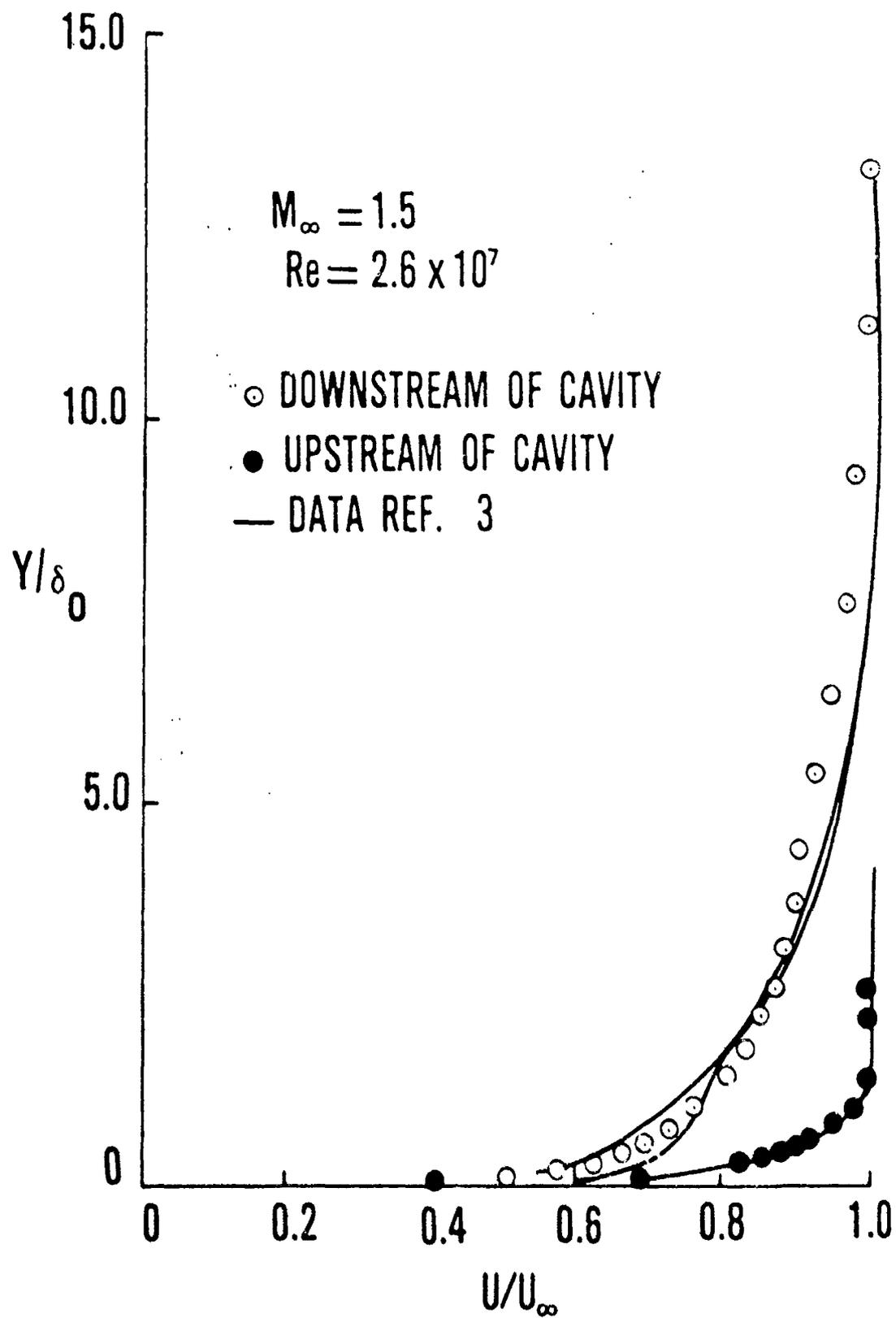
Figure 10. Comparison of Velocity Profiles
