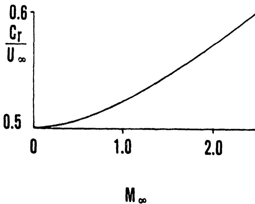
Figure 3. Propagation Velocity v.s. Mach Number of Traveling Waves in a Free Shear Layer (Ref. 12)
