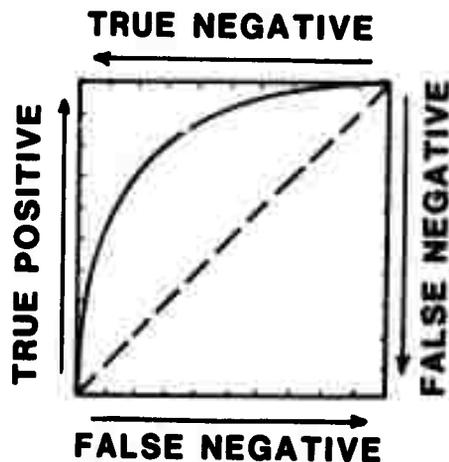
Figure 12 Typical Relative Operating Characteristic (ROC) Curve (REF 10)
