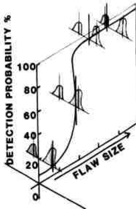
Figure 9 Interaction of Acceptance Criteria with the Probability of Detection (POD)
