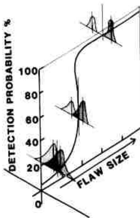
Figure 7 Interaction of Signal / Noise Discrimination with the Probability of Detection (POD)
