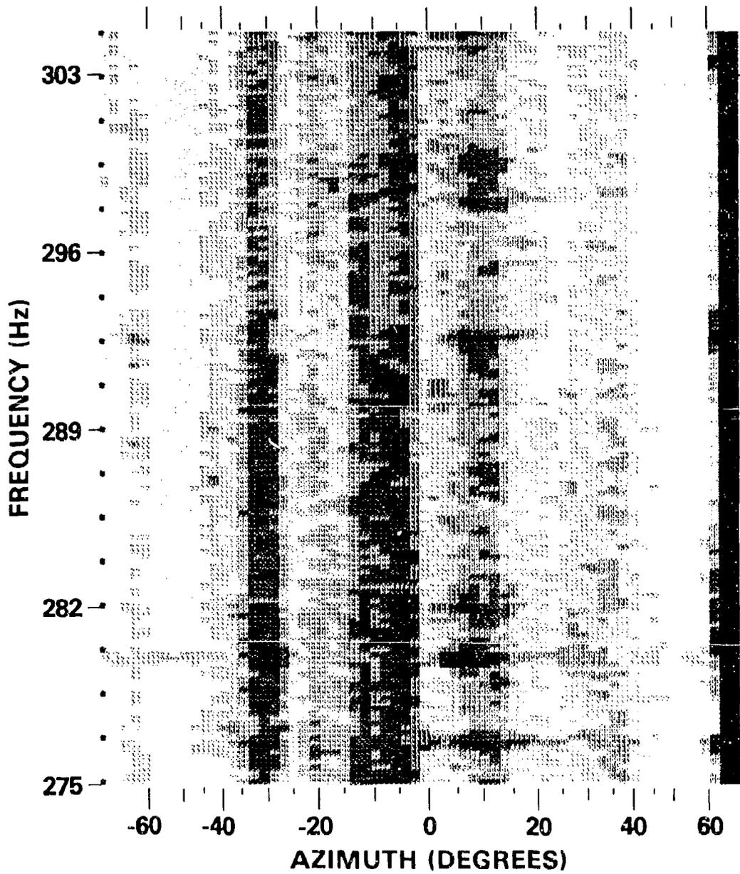
Fig. C.2 (C) — Beam power obtained using estimates for missing hydrophones, 41-59 dB/uPa IIF band, sample one (U)
