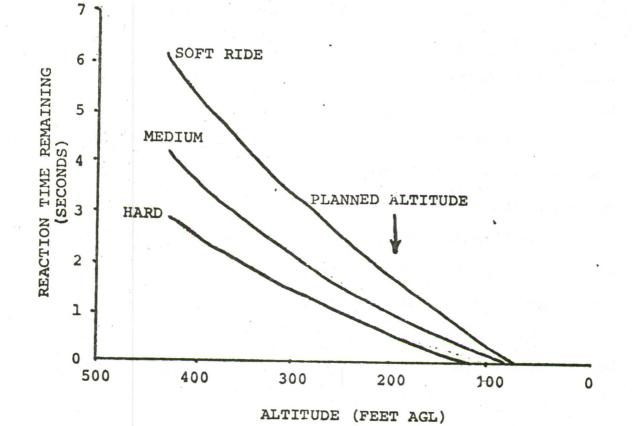
PLANNED TFR LETDOWN FROM 500' TO 200' AGL DIVE COMMAND WITHOUT 68% FLY UP NET +4g RECOVERY PULL UP RESULTS FROM GENERAL DYNAMICS FLIGHT SIMULATOR 480 KTAS
