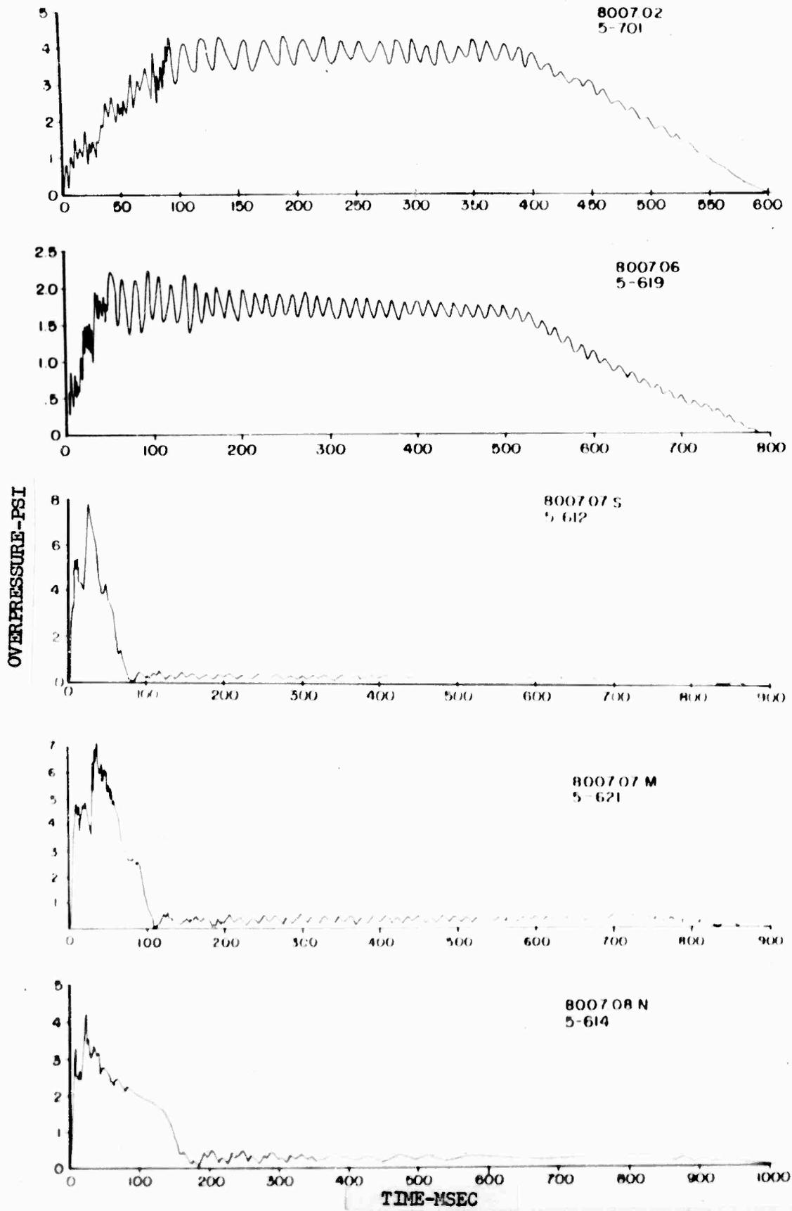
Figure B.25 Over-Pressure-Time Records, Gages Inside Valves, Sta. 31.5/7.02/7.06/7.07/7.
