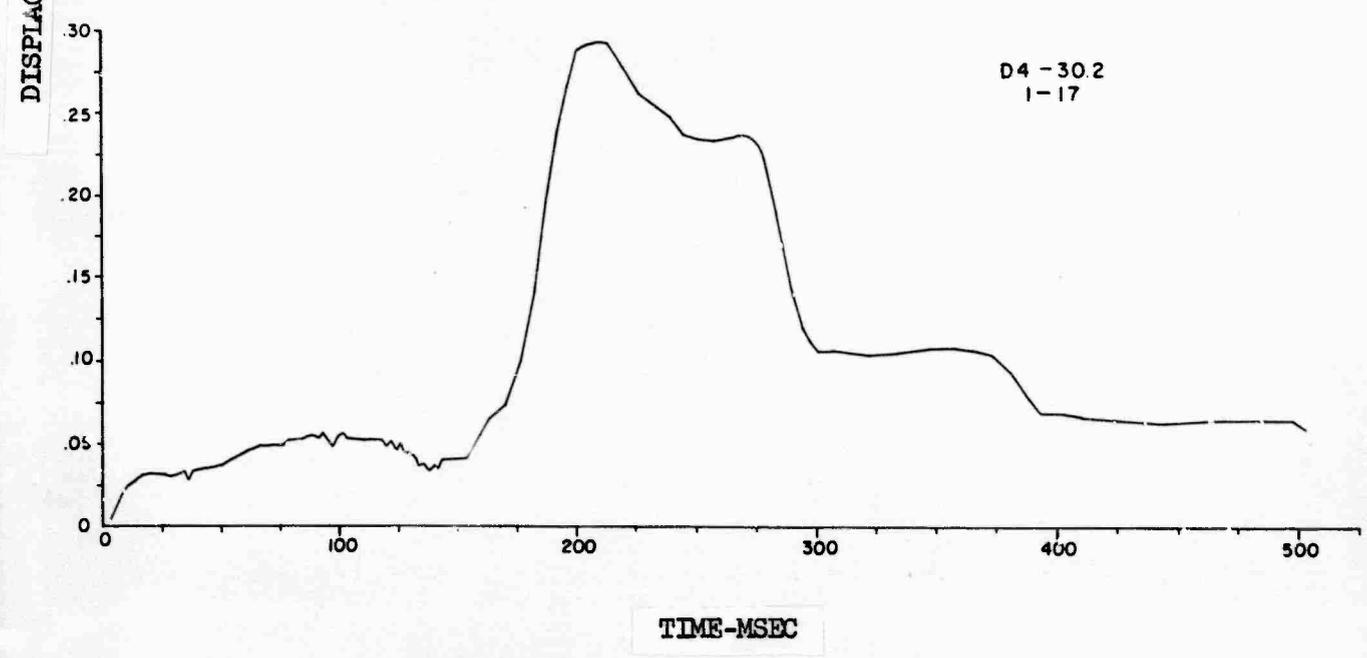
Figure B.7 Displacement-Time Record, Gage D4, Station 30.2/2.00
