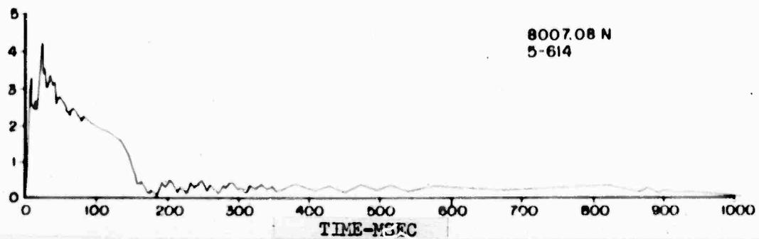
Figure B.25 Over-Pressure Time Records, Gages Inside Valves, Sta. 31.5/7.02/7.06/7.07/7
