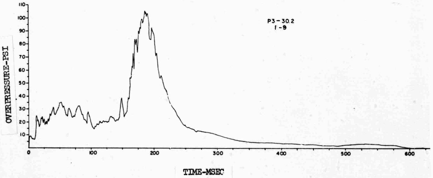
Figure B.5 Over-Pressure-time Record, Gage P3, Station 30.2/2.00
