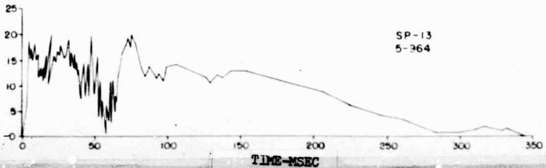
Figure B-19 Over-Pressure-time Records, Gauges SP-7 to SP-13, Station 5.6/8.01
