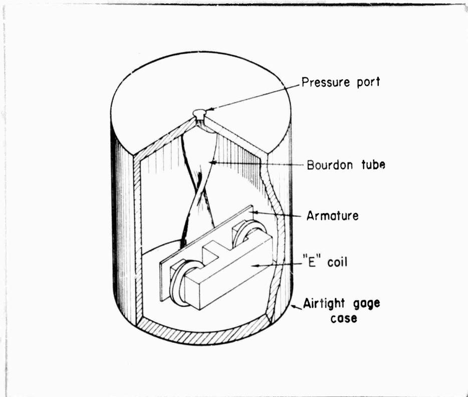
Figure 2.24 Schematic drawing of pressure-gage configuration.
