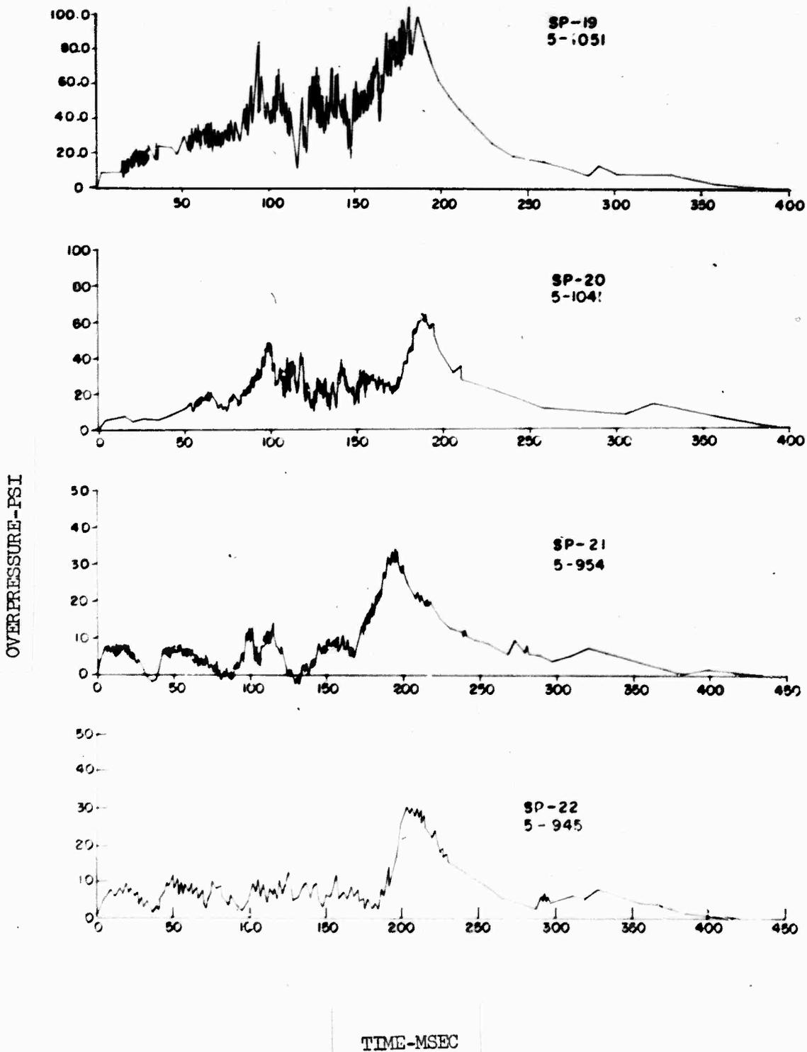
Figure B-13 Over-Pressure-Time Records, Gauges SP 19 to SP 22, Station 3.5/7.02
