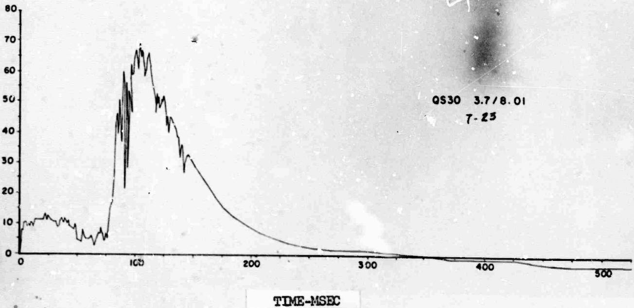
Figure B.2 Side-On Over-Pressure-Time Record, Gage QS30, Station 3.7/8.01
