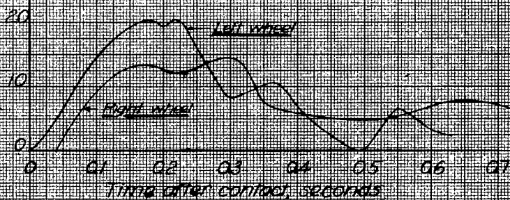
Figure 18—Time history of wing and center of gravity acceleration and landing gear normal load in a normal landing. Vertical velocity 2.4 fps. Landing 17, B-24D airplane.
