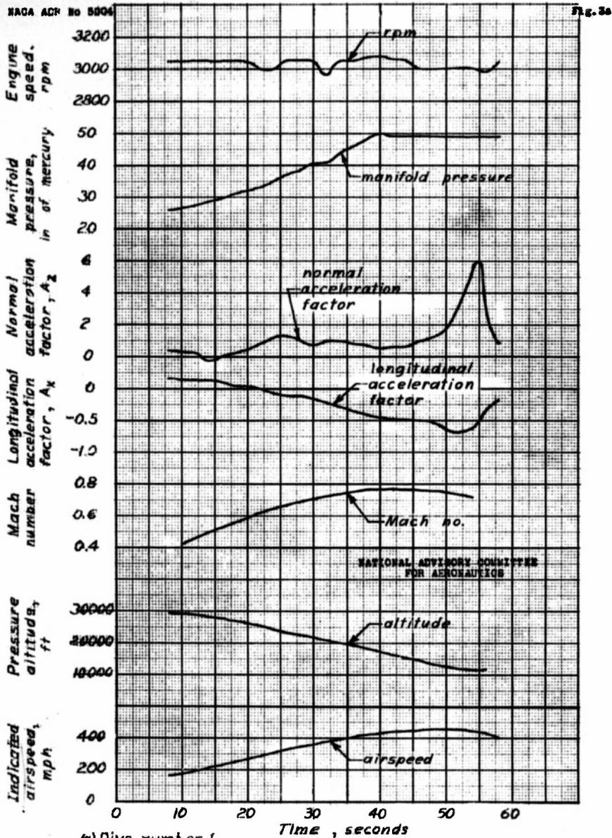
Figure 3- Time history of a power-on dive from 30,000 feet. Clean condition, oil and coolant shutters flush. Bell P-39N-1 airplane.
