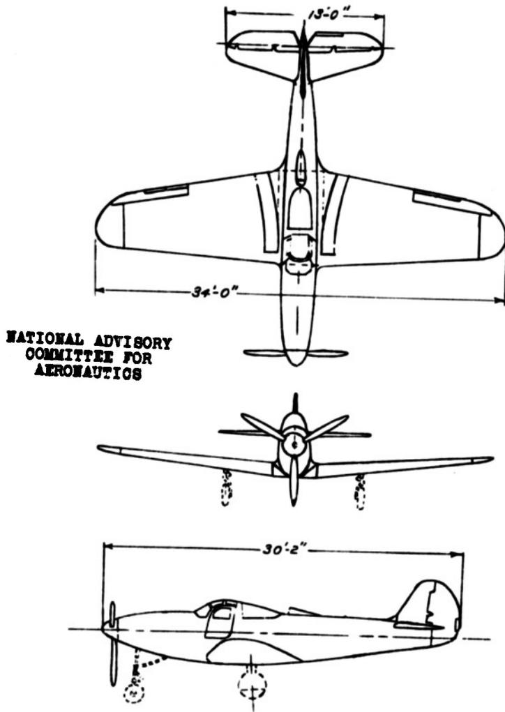
Figure 1.- Three-view drawing of the Bell P-39N-1 airplane.
