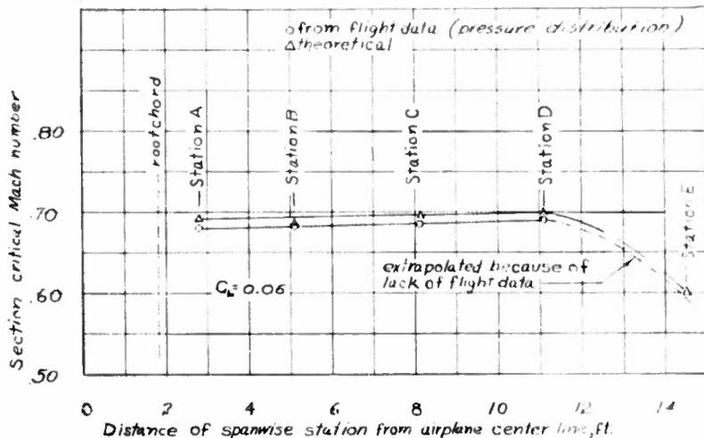
Figure 8- Variation of section critical Mach number with span on the P-39N-1 airplane.
