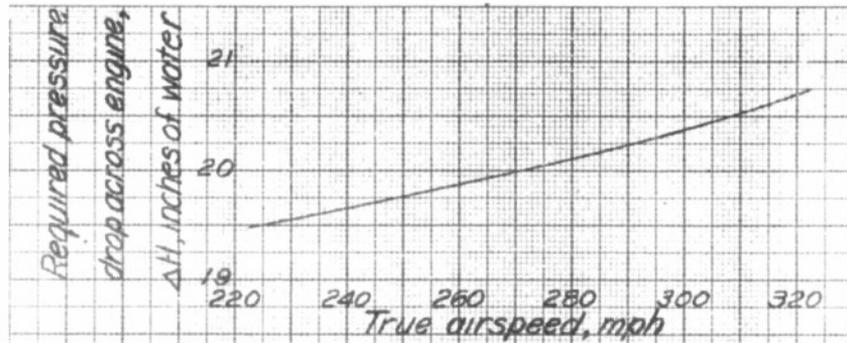
Figure 22.-Variation of required pressure drop across engine with airspeed. Engine operating at cruise rating of 1200 bhp at 2100 rpm; altitude, 14,000 feet.
