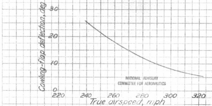
Figure 23.-Variation of required cowling-flap deflection with airspeed. Conventional engine-cooling system; engine operating at cruise rating of 1200 bhp at 2100 rpm; altitude, 14,000 feet.
