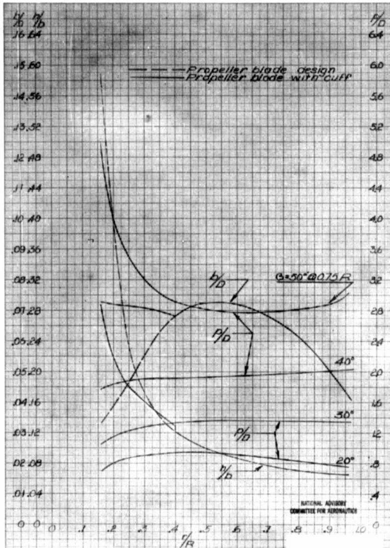
Figure 6. Blade form curves for Hamilton Standard propeller 6457A-6 with cuffs.  $D$ , diameter;  $R$ , radius to tip;  $b$ , section chord;  $h$ , section thickness;  $p$ , geometric pitch of section chord line.
