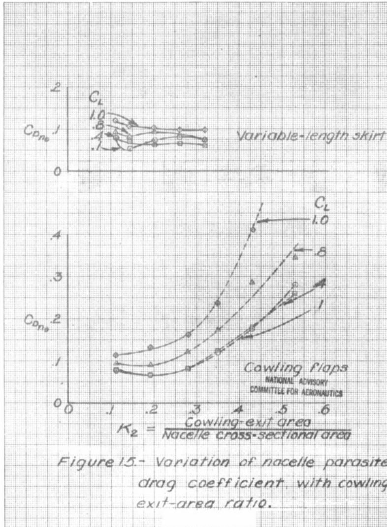
Figure 15.- Variation of nacelle parasite drag coefficient with cowling-exit-area ratio.
