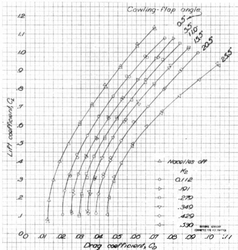
Figure 12.- Comparison of lift & drag characteristics of airplane model showing effect of nacelle and of cowling-flap deflections.
