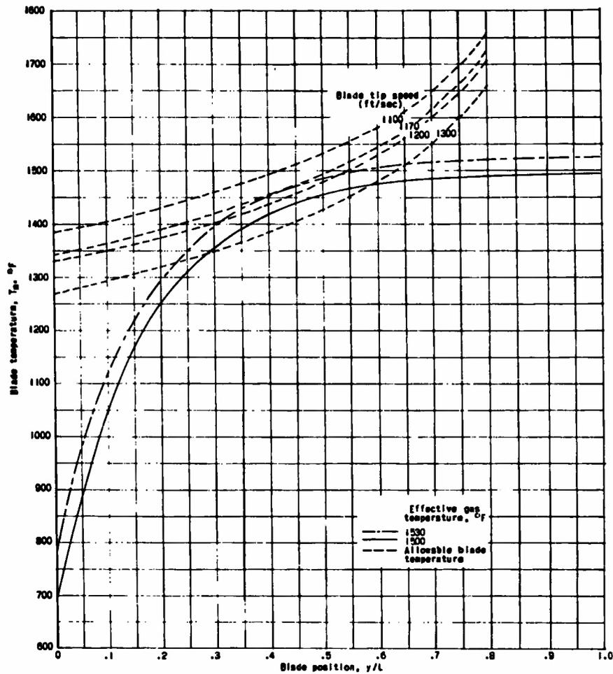
Figure 5. - Allowable Increase in effective gas temperature for turbine with cooling fins on the rim. Blade tip speed, 1170 feet per second; blade life, 1000 hours.
