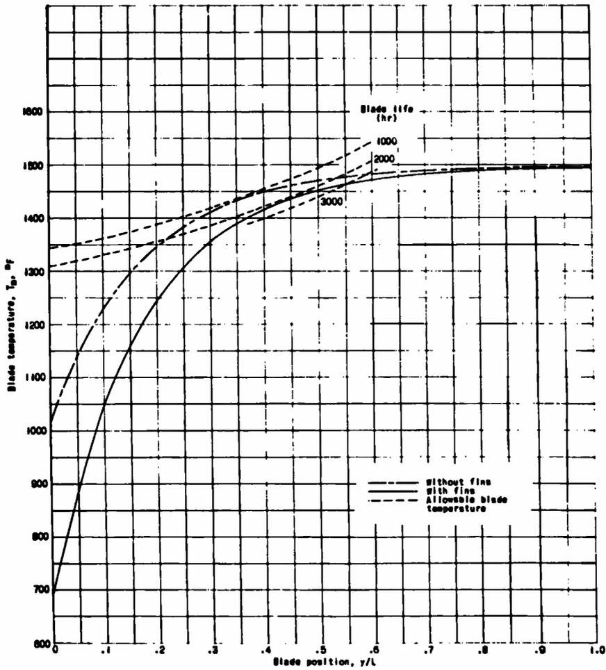
Figure 4. - Allowable increase in blade life for turbine with cooling fins on the rim for blade tip speed of 1170 feet per second and effective gas temperature of 1500° F.
