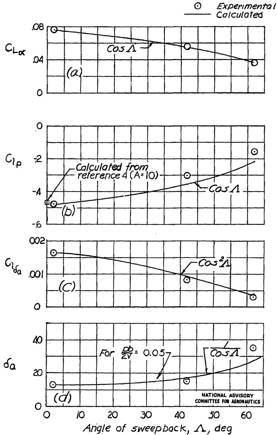
Figure 8 - Comparison of calculated and experimental values of  $C_{L\alpha}$ ,  $C_{l_p}$ ,  $C_{l_{\delta a}}$ , and  $\delta_a$  for three wings with  $2^\circ$ ,  $42^\circ$ , and  $62^\circ$  sweepback.  $C_L = 0.3$ .
