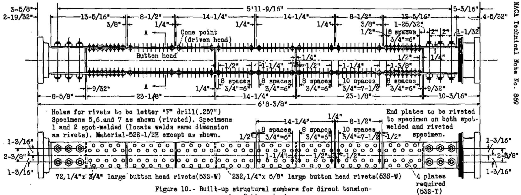
Figure 10.- Built-up structural members for direct tension-compression fatigue tests.
