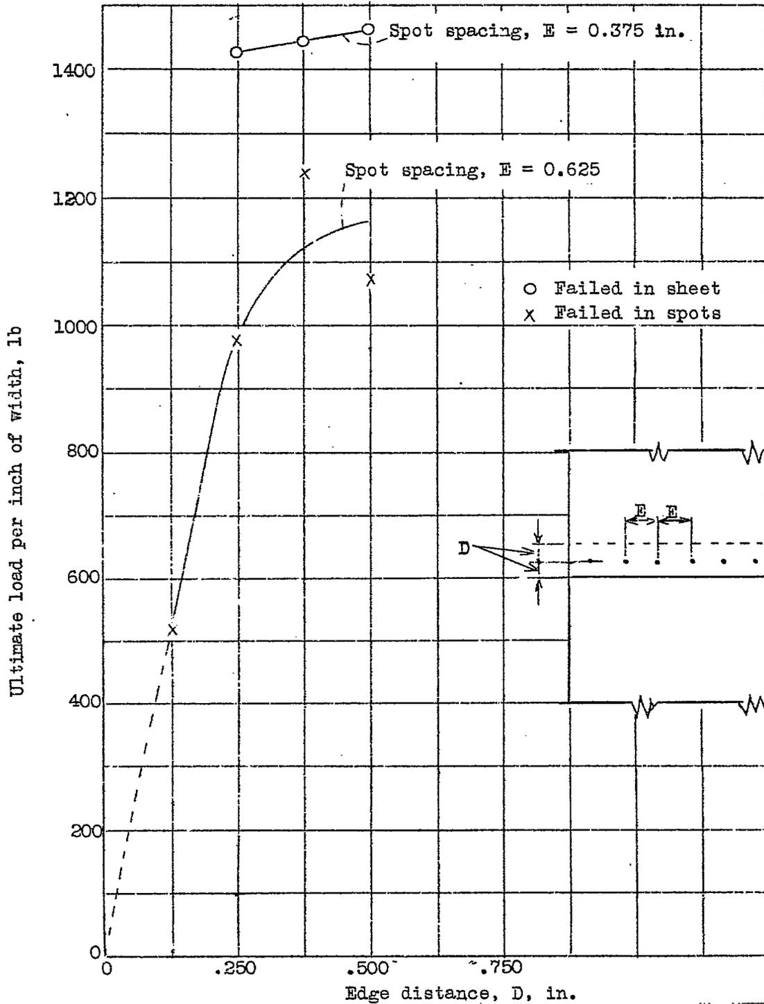
Figure 4.- Effect of edge distance on strength of spot-welded joints in .051-inch thick 52S-1/2H sheet.
