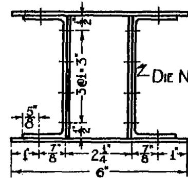
Hole diameter for riveted beams,  $\frac{17}{64}$  inches
