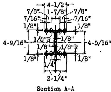
Figure 11.- Direct tension-compression fatigue tests of spot-welded and riveted structural members. Sheet, 52S-1/2H; ratio of minimum stress to maximum stress, -1.0.
