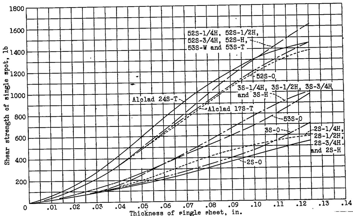
Figure 1.- Minimum shear strength of spot welds.
