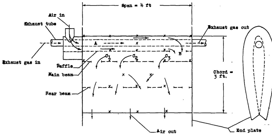
Figure 3.- Set-up of wing heated by exhaust tube, showing path of exhaust gas and air through the model and the location of skin-temperature thermocouples, x.
