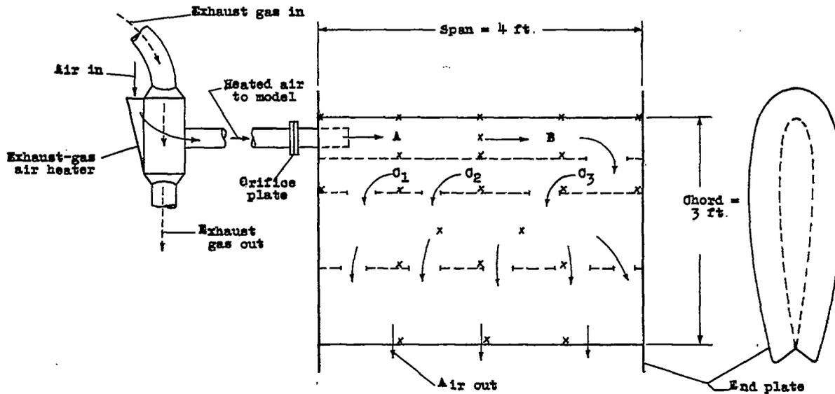
Figure 4.- Set-up of wing heated by hot air, showing path of heated air through the model and the location of skin-temperature thermocouples.
