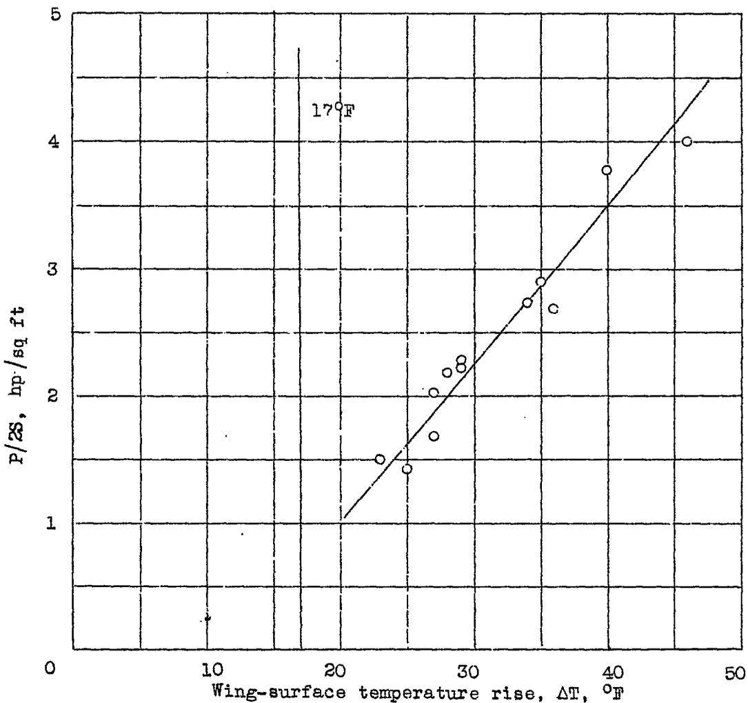
Figure 9.- The calculated temperature rise for 12 modern transport airplanes. (17°F is temperature rise required for ice prevention at 15°F )
