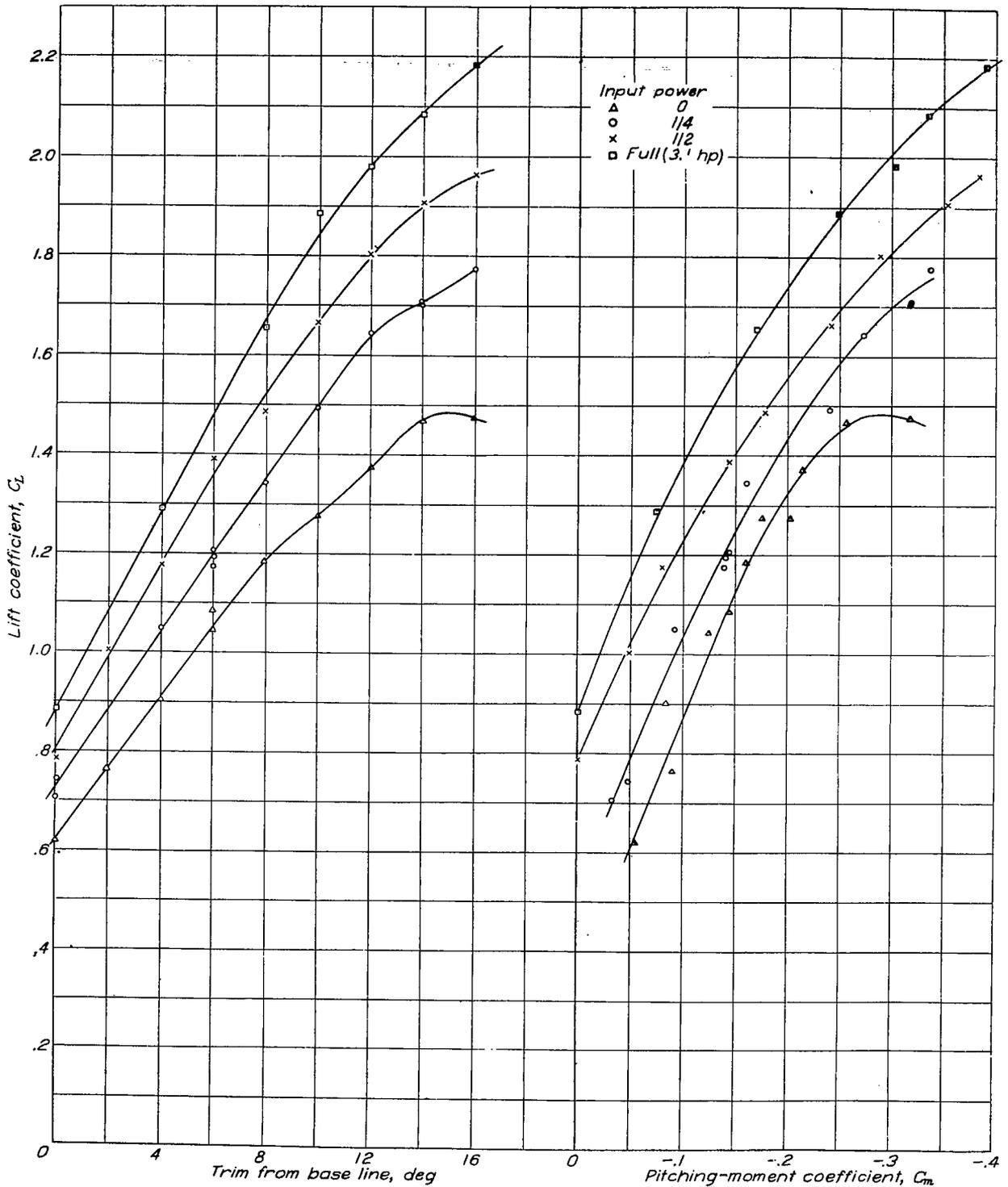
Figure 4.- NACA model 117 with power. Results of aerodynamic tests with flaps down  $30^\circ$ , stabilizer down  $5^\circ$ , elevators neutral.  $C_m$  referred to center of gravity at 22.6 percent M.A.C. Height of center of gravity was such that afterbody was just clear of water at  $16^\circ$  trim.
