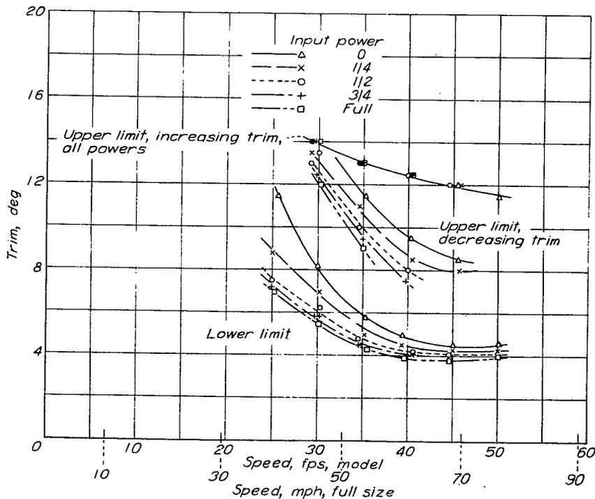
Figure 6.- NACA model 117. Effect of power on limits of stability. Flaps down 30°.
