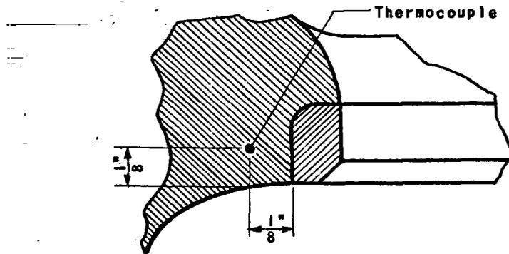
(a) Section through valve seat.
