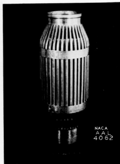
Figure 14.- Heat exchanger 6 as installed in the B-17F airplane. Weight as shown, 34.3 pounds.
