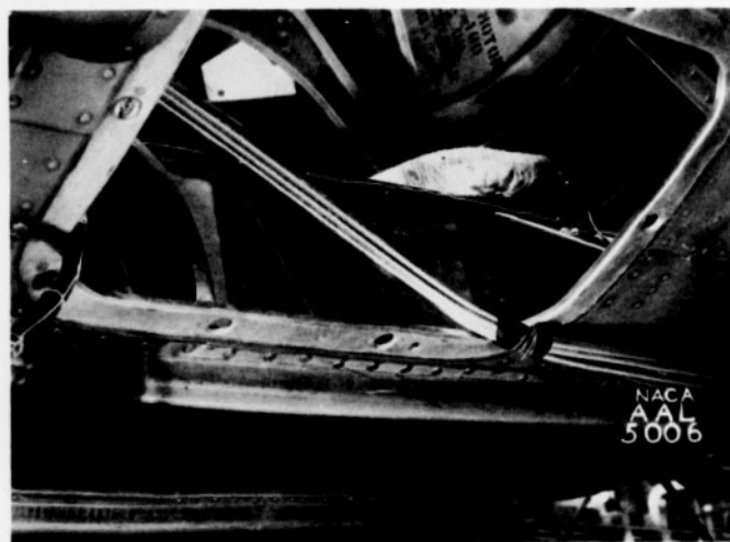
Figure 23.- Nacelle 4 exhaust shroud as altered for installation of heat exchangers 3, 4, and 5. B-17F airplane.
