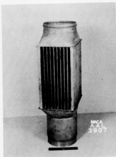
Figure 8. Heat exchanger 3 as installed in the B-17F airplane. Weight as shown, 29.0 pounds.
