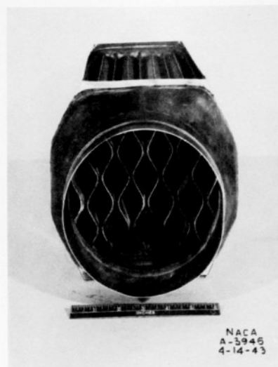
Figure 12.- Heat exchanger 5. Air inlet and outlet openings were slightly enlarged when installed in the B-17F airplane. Weight as shown, 33.0 pounds.
