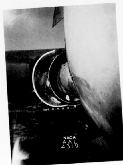
Figure 36.- Heat exchanger 7 installation in nacelle 3, ready for flight. B-17F airplane.
