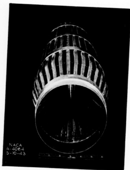
Figure 17.- Heat exchanger 7 as installed in the B-17F airplane. Weight as shown, 51.3 pounds.
