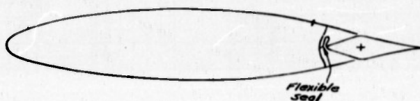
Figure C87: Schematic view of the internally balanced and sealed aileron on low-drag wing of Curtiss XP-60.
