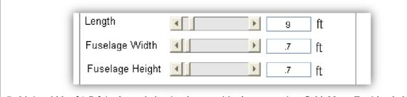
Robin's width of 0.7 ft is shown being implemented in the appropriate field. Note: For blended wing or flying wing concepts such as the aircraft shown below, use a width of 1/3 the wingspan.
