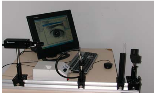
Figure 4. Laboratory system designed for iris recognition tests.
