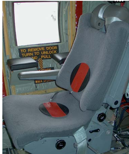
b. ARWO Seat Pan and Seat Back Accelerometer Pads
