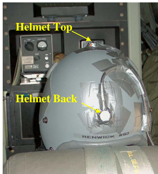
c. ARWO Helmet Top and Helmet Back Accelerometer Packs
