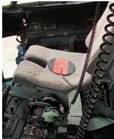
f. Copilot Seat Pan Accelerometer Pad
