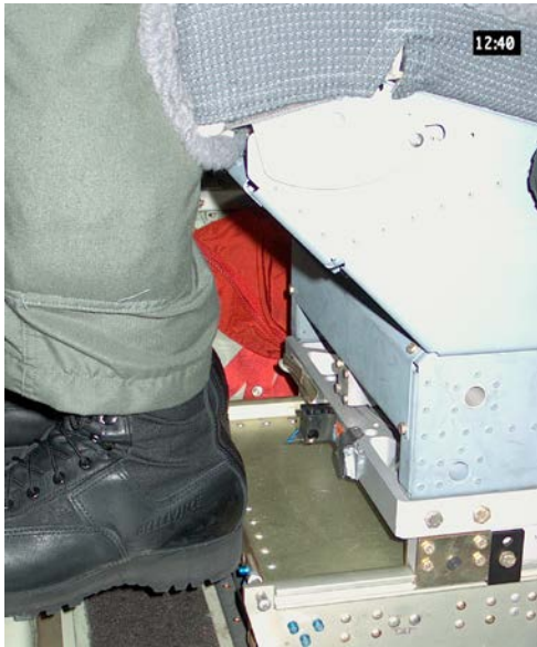
a. ARWO Seat Base Accelerometer Pack
