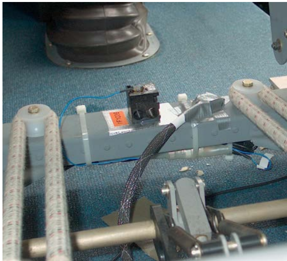
e. Copilot Seat Base Accelerometer Pack (located on lower front seat cross-beam)
