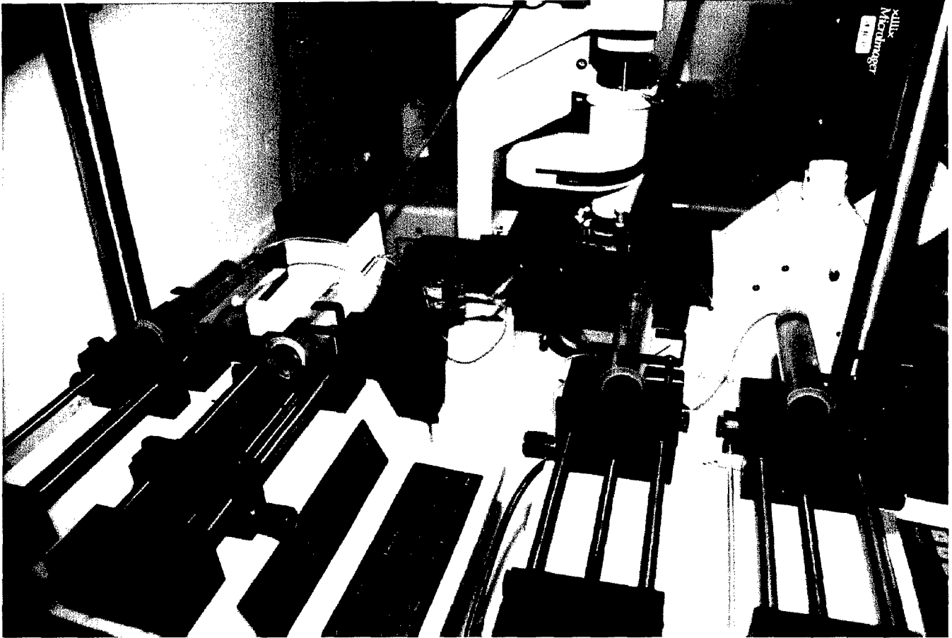
VSOM: Zeiss Inverted Fluorescence Microscope with Four Computer-Controlled Syringe Pumps leading to a temperature-controlled micro-perfusion chamber mounted on a computer-controlled xy scanning stage.
