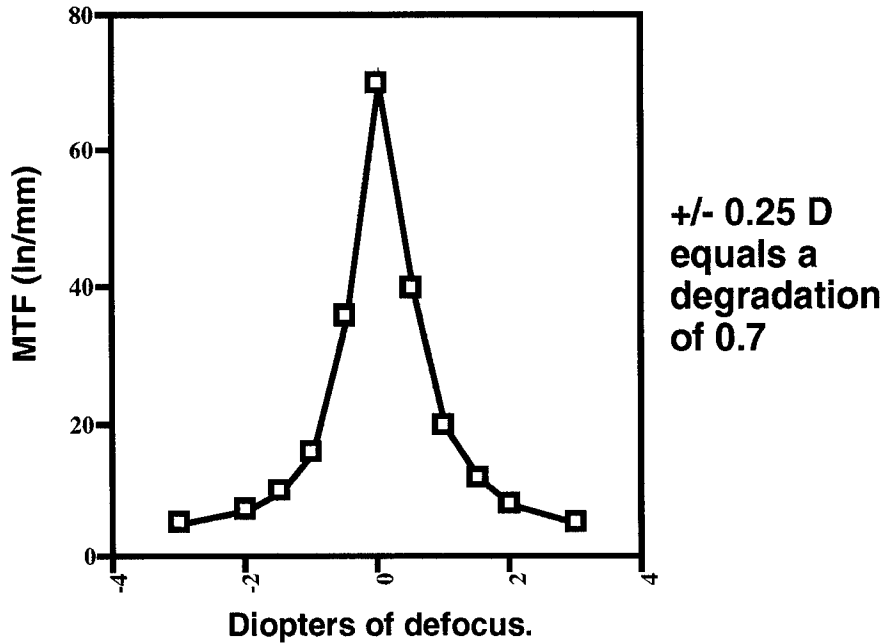
Fig. 8. MTF reduction vs. focal error.
