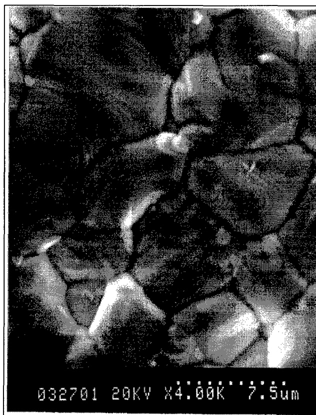
Figure 10. SEM surface view of a pure Ag electrode on the YSB electrolyte.
