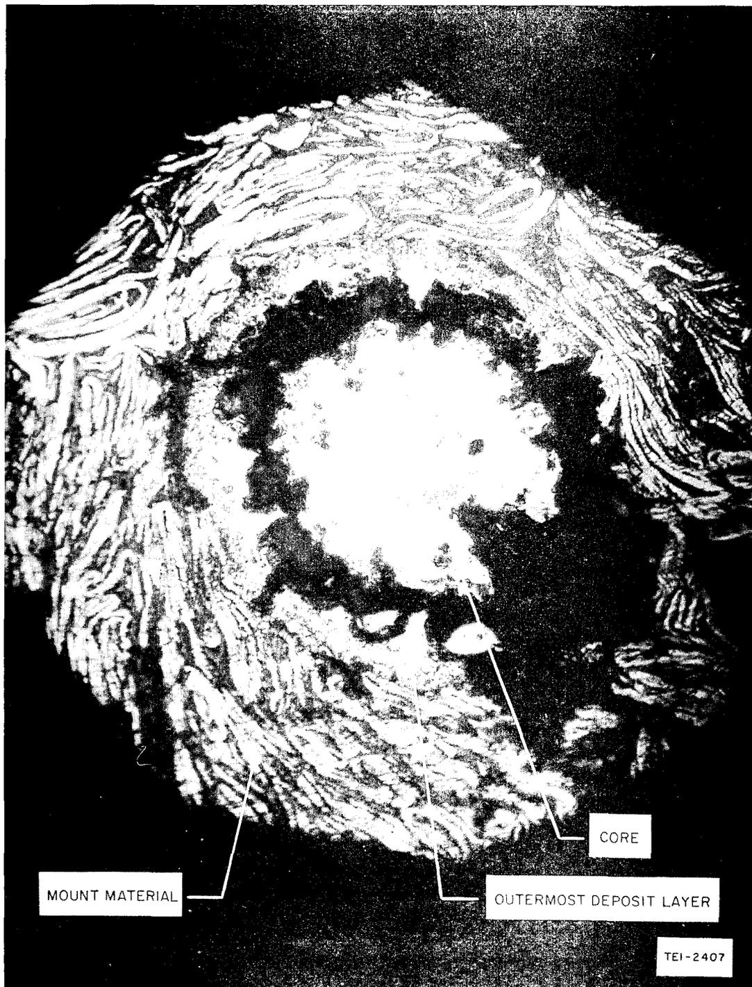
Fig. 20 Photomicrograph of Cross-Section of  $TiB_2$  Fiber Heated to  $1800^\circ C$  for 45 Minutes
