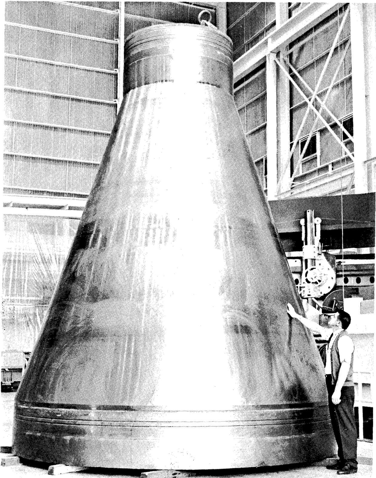
Figure 6 - Mandrel for Wrapping of Exit Cone
