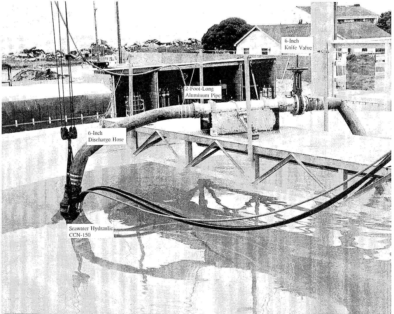
Figure 7 Full scale test setup.
