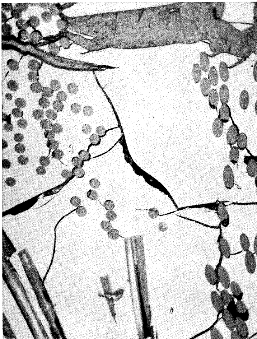
Figure 14 1000°F OVEN-CHARRED SILICA-PHENOLIC MXS-89 CORING (500X MAGNIFICATION)
