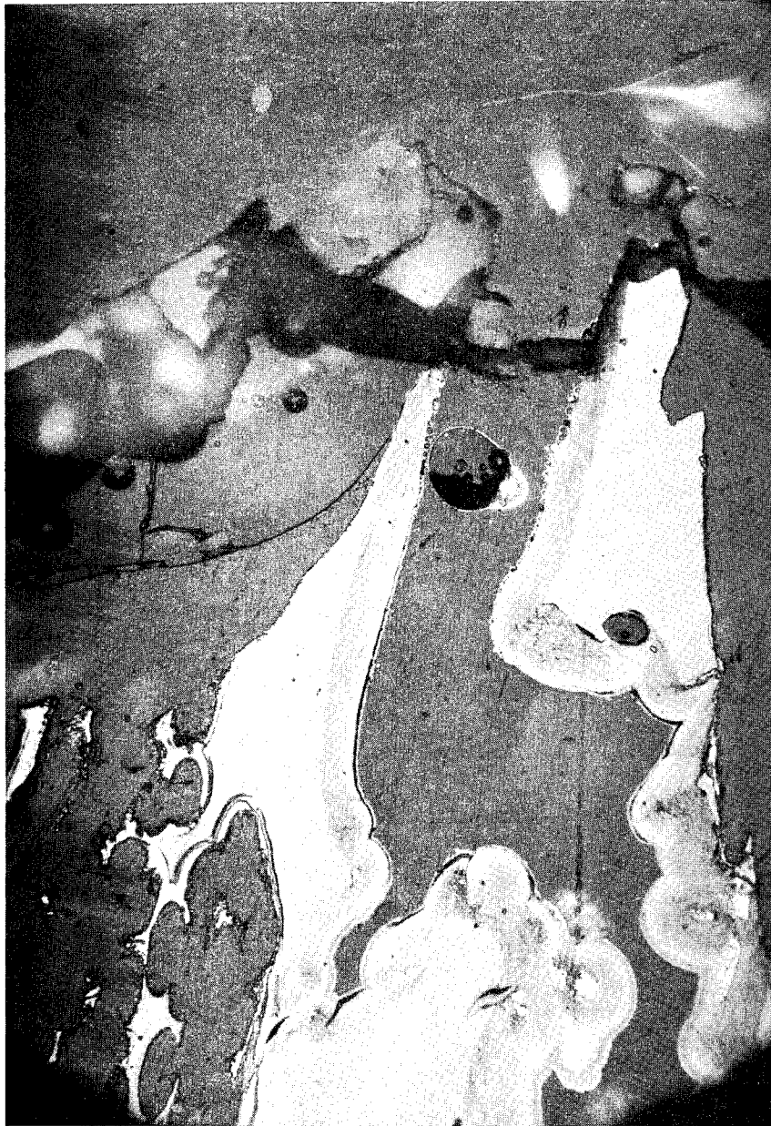
Figure 74 POST-FIRED SILICA-PHENOLIC MXS-89 NOZZLE SURFACE CHAR (500X MAGNIFICATION)
