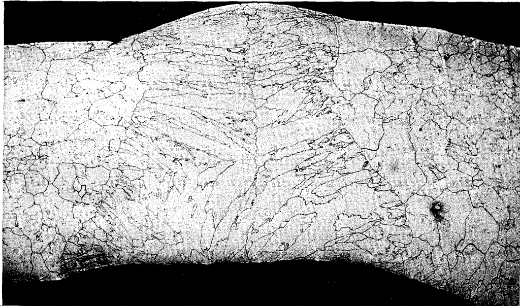
Figure H-3. Microstructure of Tank Weld Adjacent to Fracture (Liner material at left, weld nugget center, and boss right. Note the coarse grain structure in the heat-affected zone and the directional grain orientation in the weld nugget.)
