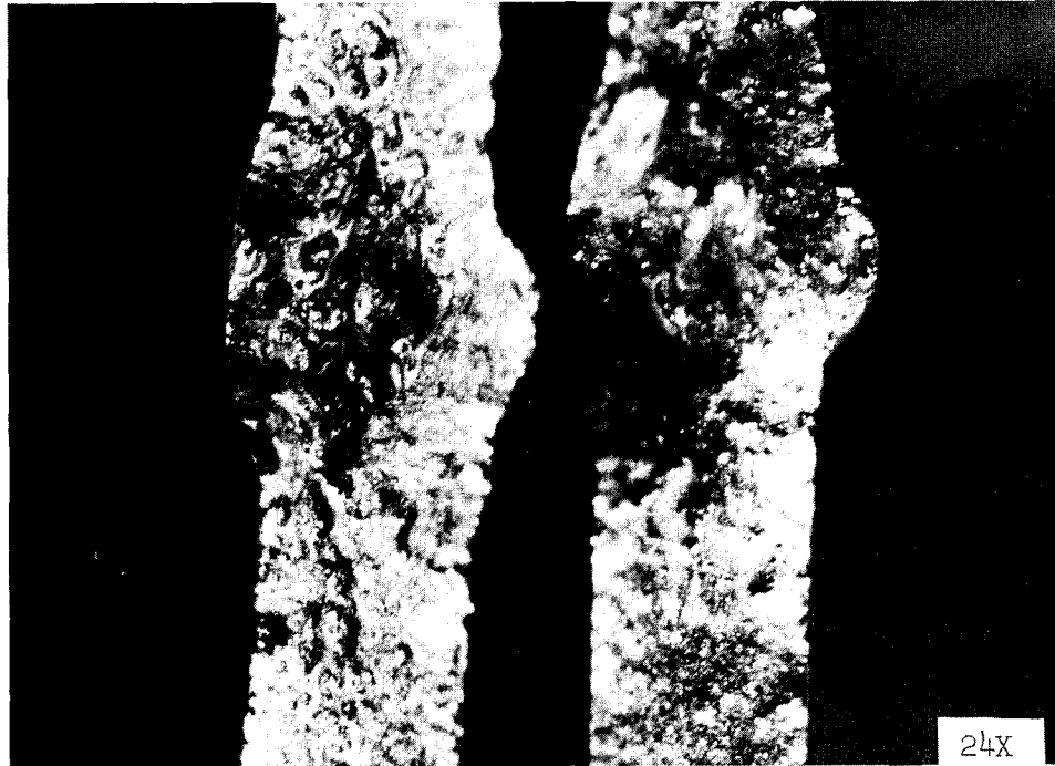
Figure H-6. Macrophotographs of Tensile Specimen L-6 (Note: Near left edge of each piece, in weld nugget, is a gas hole, photographed as a black circle.)
