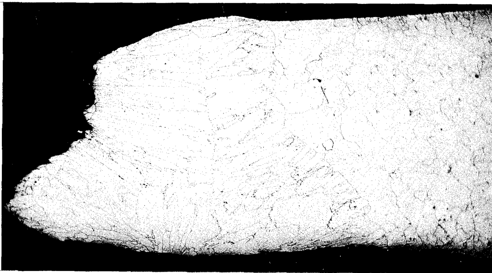
Figure H-4. Microstructure of Weld Nugget and Location of Fracture in Tank (Fracture occurred along interface between metal liner and weld nugget.)
