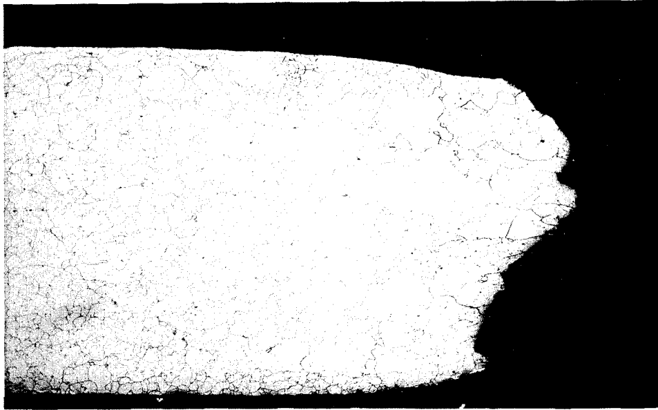
Figure H-5. Microstructure of Metal Liner (Note that the heat-affected-zone grain structure is coarser than the rest of the parent material.)
