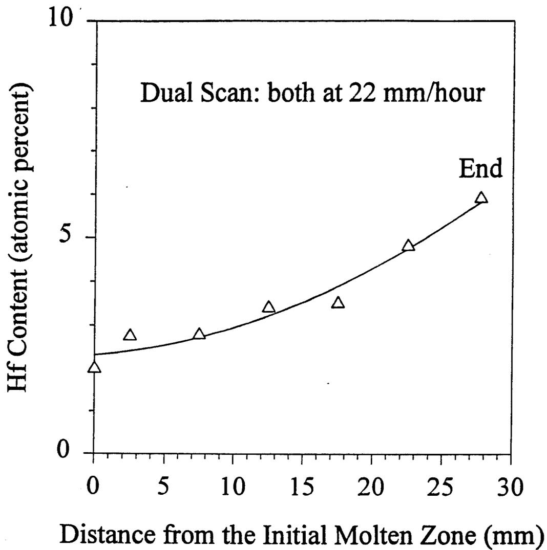
Figure 23. The composition profile in a Mo-3.71% Hf-1% C single crystal.
