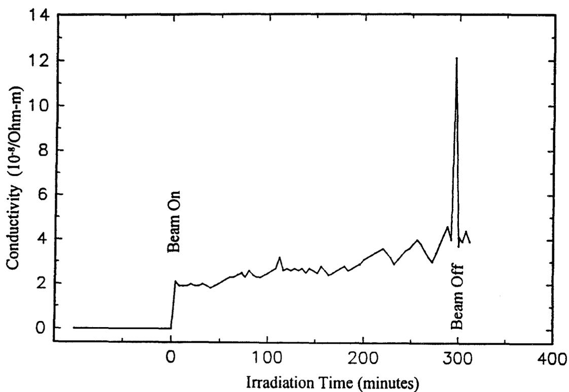
Figure 5. Radiation induced conductivity in polycrystalline alumina irradiated with 2 MeV alpha at 673 K at an average beam current density of 800 nA/cm<sup>2</sup>.
