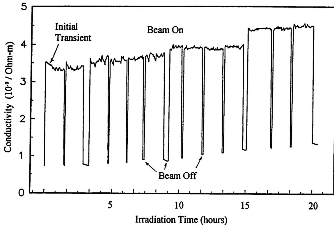
Figure 6. Effects of proton irradiation on the conductivity of sapphire.
