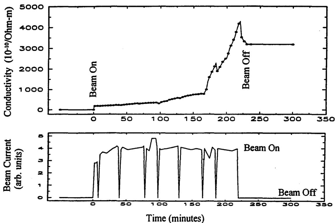
Figure 3. Radiation induced conductance in polycrystalline alumina irradiated with 2 MeV protons at 673 K at an average beam current density of 800 nA/cm<sup>2</sup>. Same as figure 2 but irradiated four times as long in duration (also a new sample).
