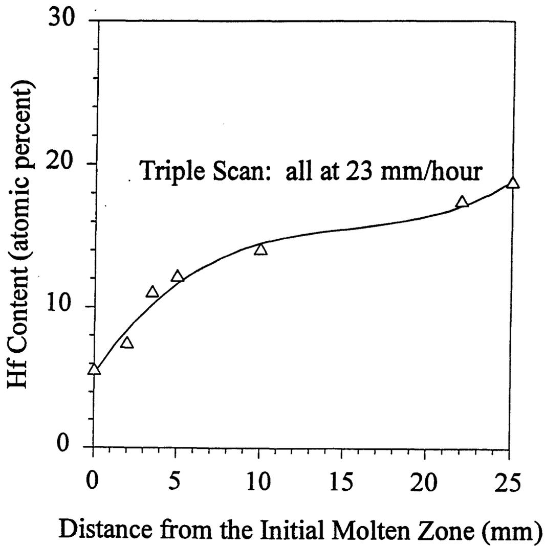
Figure 24. The composition profile in a polycrystalline Mo-10%Hf-2%C sample.
