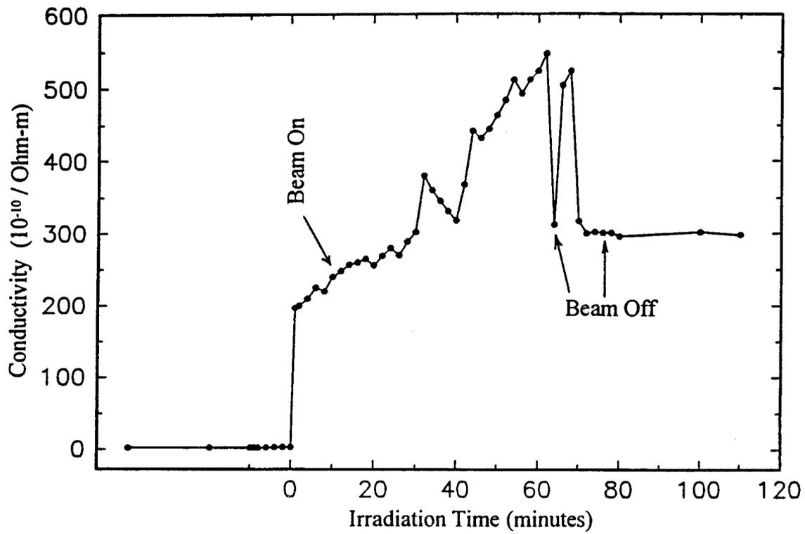
Figure 2. Radiation induced conductance in polycrystalline alumina irradiated with 2 MeV protons at 673 K at an average beam current density of 800 nA/cm<sup>2</sup>.
