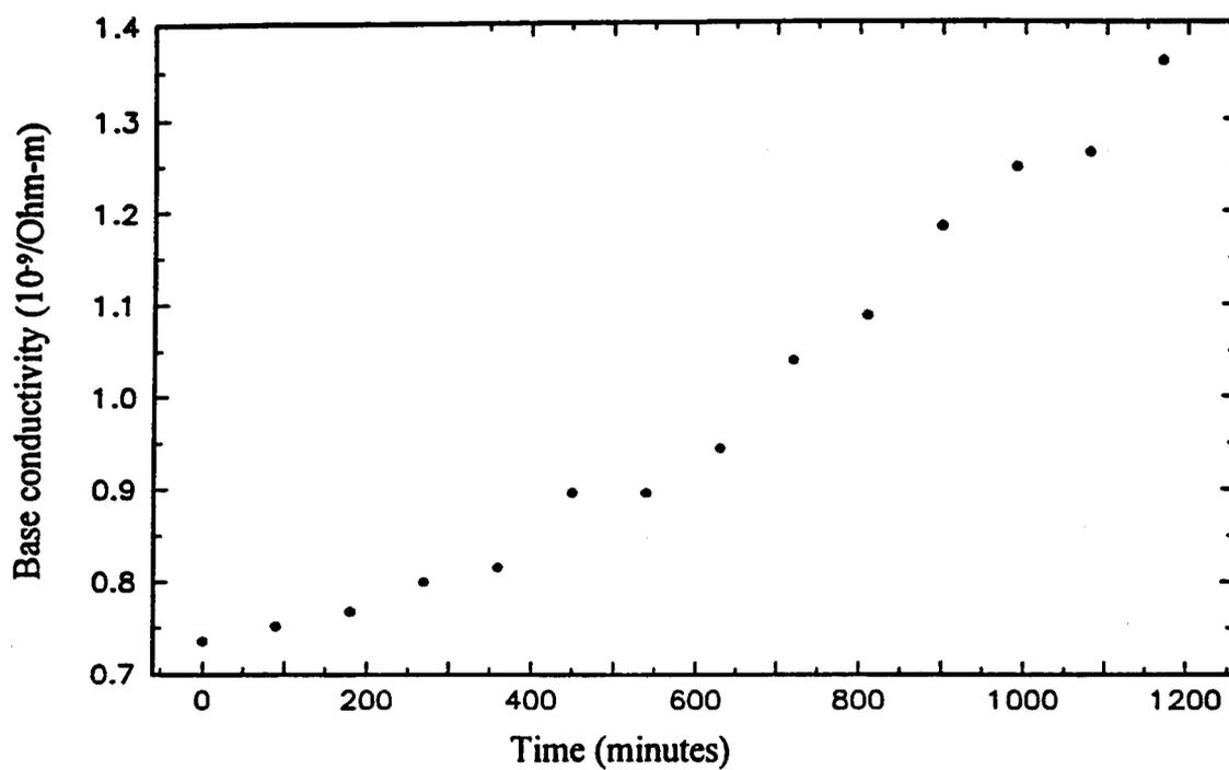
Figure 7. The change of base conductivity of sapphire as a function of irradiation time for the sample shown in figure 6.
