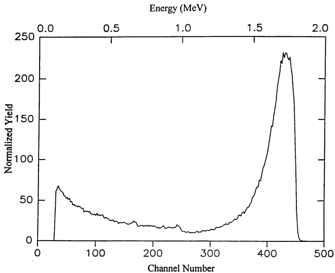
Figure 12. Same as figure 10 but for polycrystalline alumina, showing extensive inward diffusion of the deposited gold layer.
