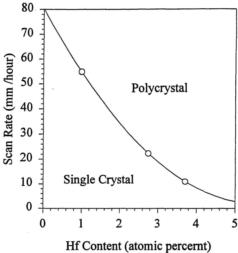
Figure 20. Experimentally determined maximum scan rate (dual scan) as a function of hafnium content required for forming Mo-Hf alloy single crystals.
