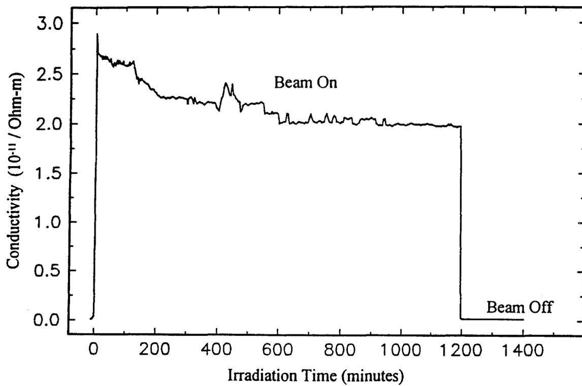
Figure 8. Effect of gamma radiation on the conductivity of sapphire.
