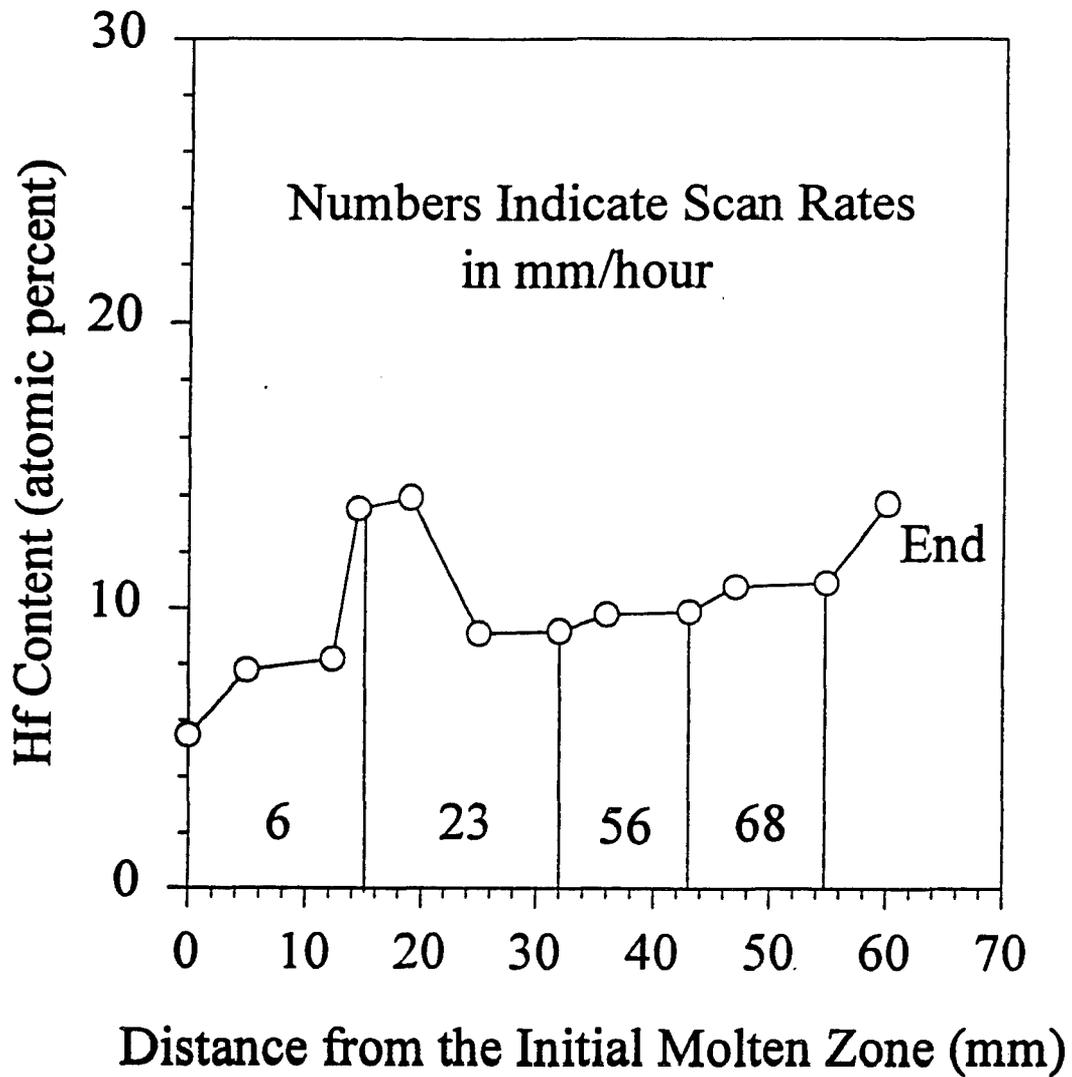
Figure 21. The composition profile in a polycrystalline Mo-10%Hf-2%C sample after first scan.
