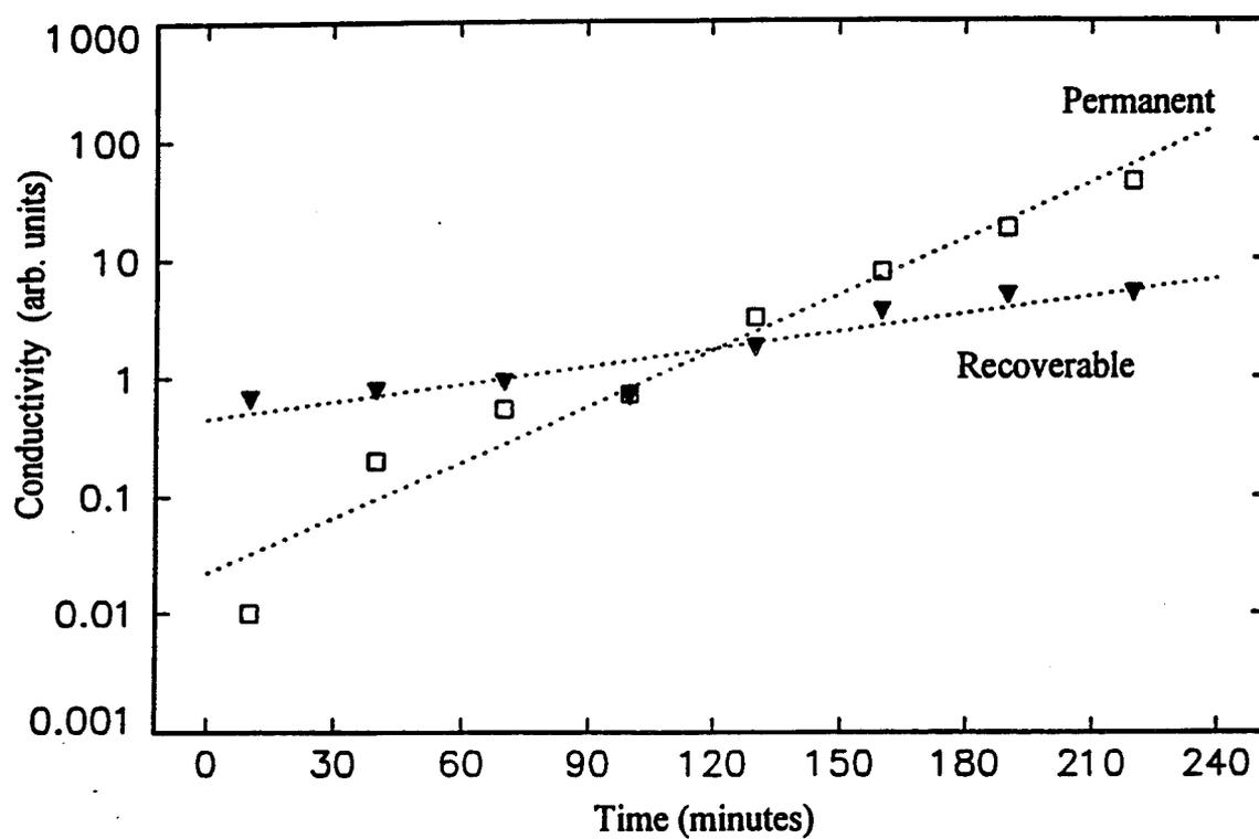
Figure 4. Effects of proton irradiation on recoverable and permanent conductivity. The lines represent best fits to the data using a linear regression method.
