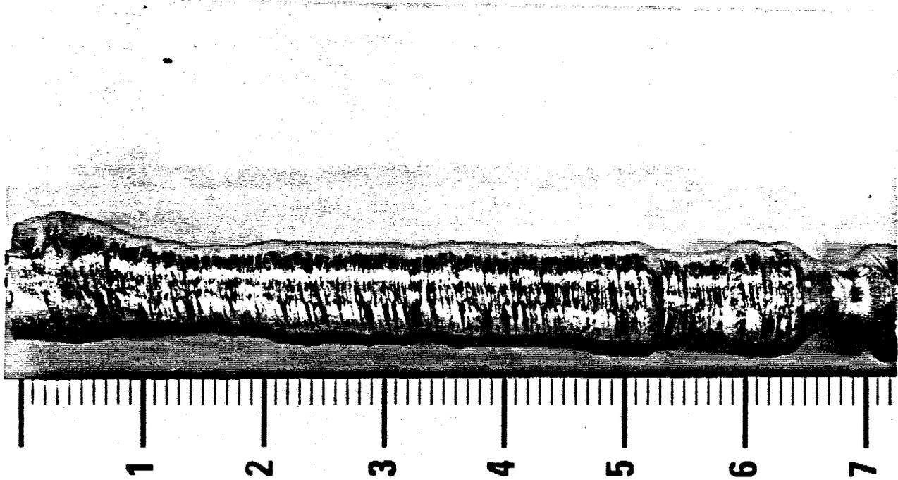
Figure 15. The surface morphology of an as-grown polycrystalline Mo-2%Hf (scale is centimeter).
