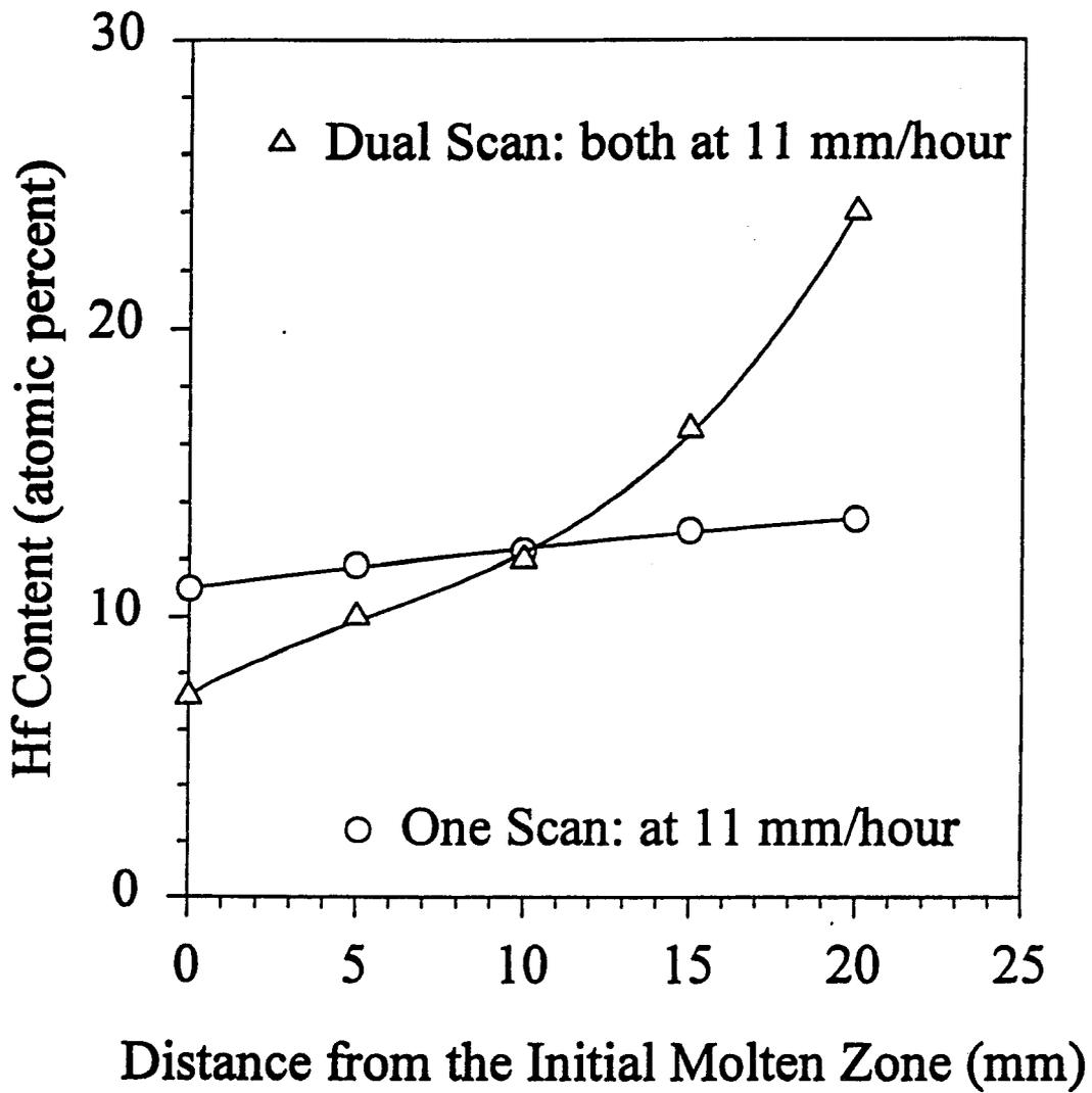
Figure 22. The composition profile in a polycrystalline Mo-15%Hf sample.
