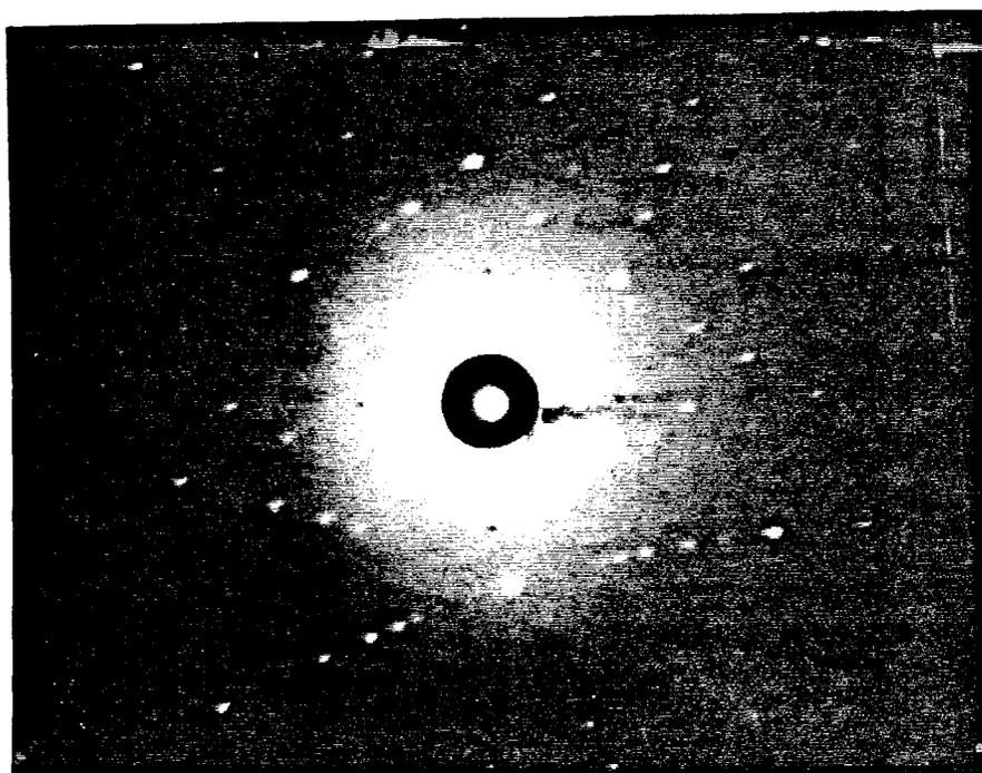
Figure 18. Laue pattern taken from the cross section of a Mo-2% Hf single crystal.
