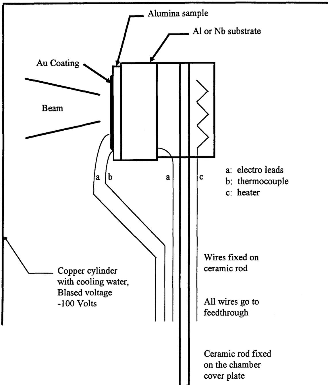
Figure 1. Schematic drawing showing the design of the sample holder for irradiation.
