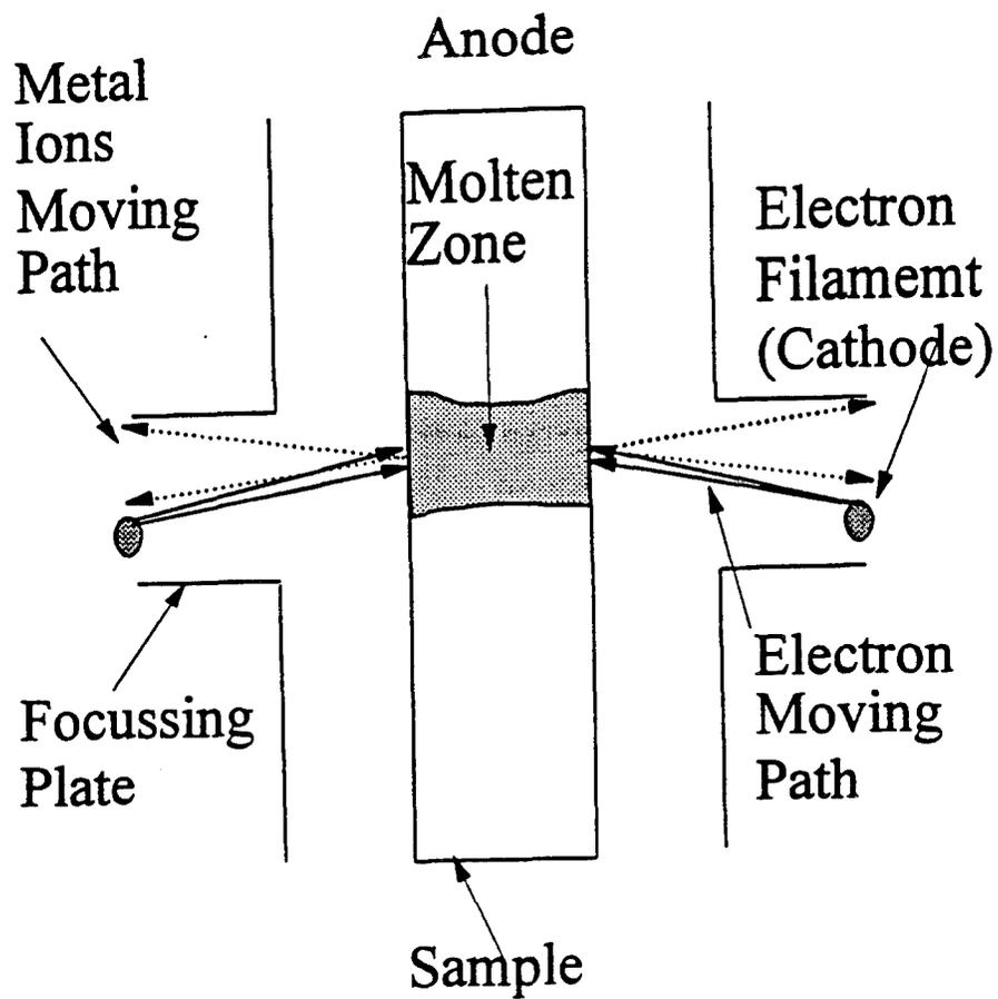
Figure 13. Schematic drawing showing the design of the electron beam gun used in this study.
