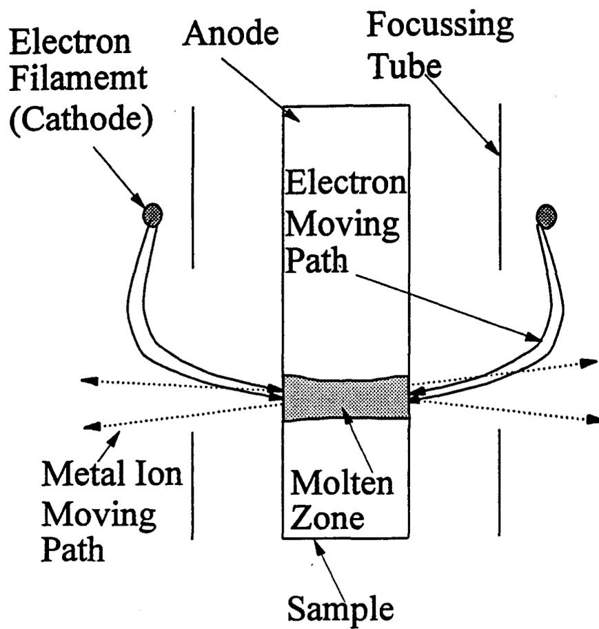
Figure 26. Schematic drawing showing the design of the improved electron beam gun.
