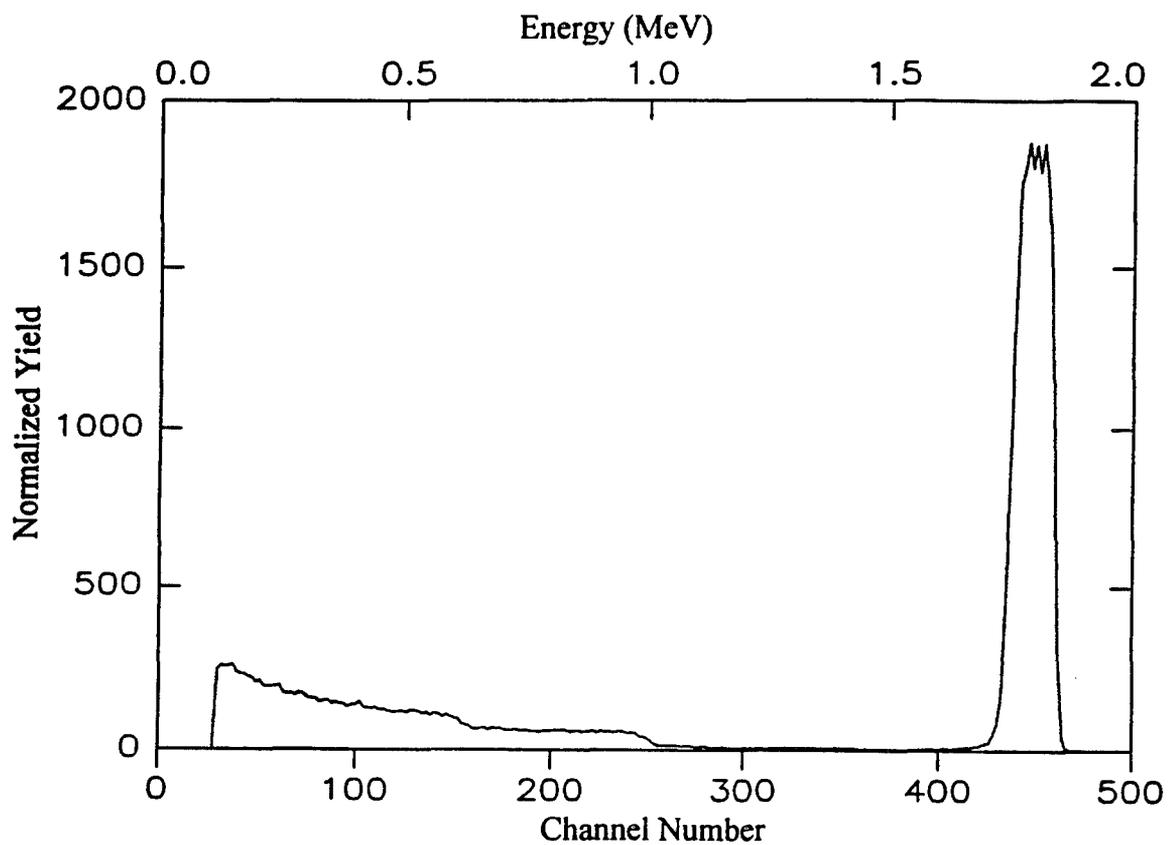
Figure 10. RBS spectrum obtained for alumina prior to irradiation.
