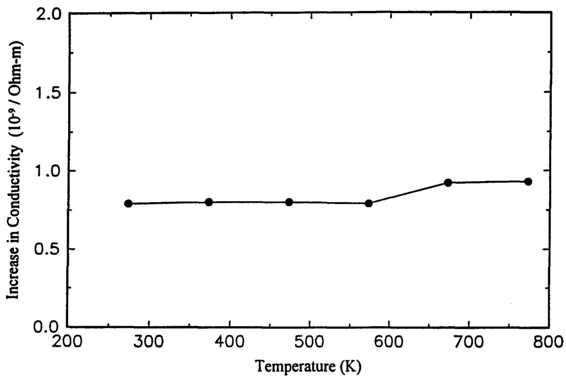
Figure 9. Temperature dependence of gamma induced conductivity in alumina.
