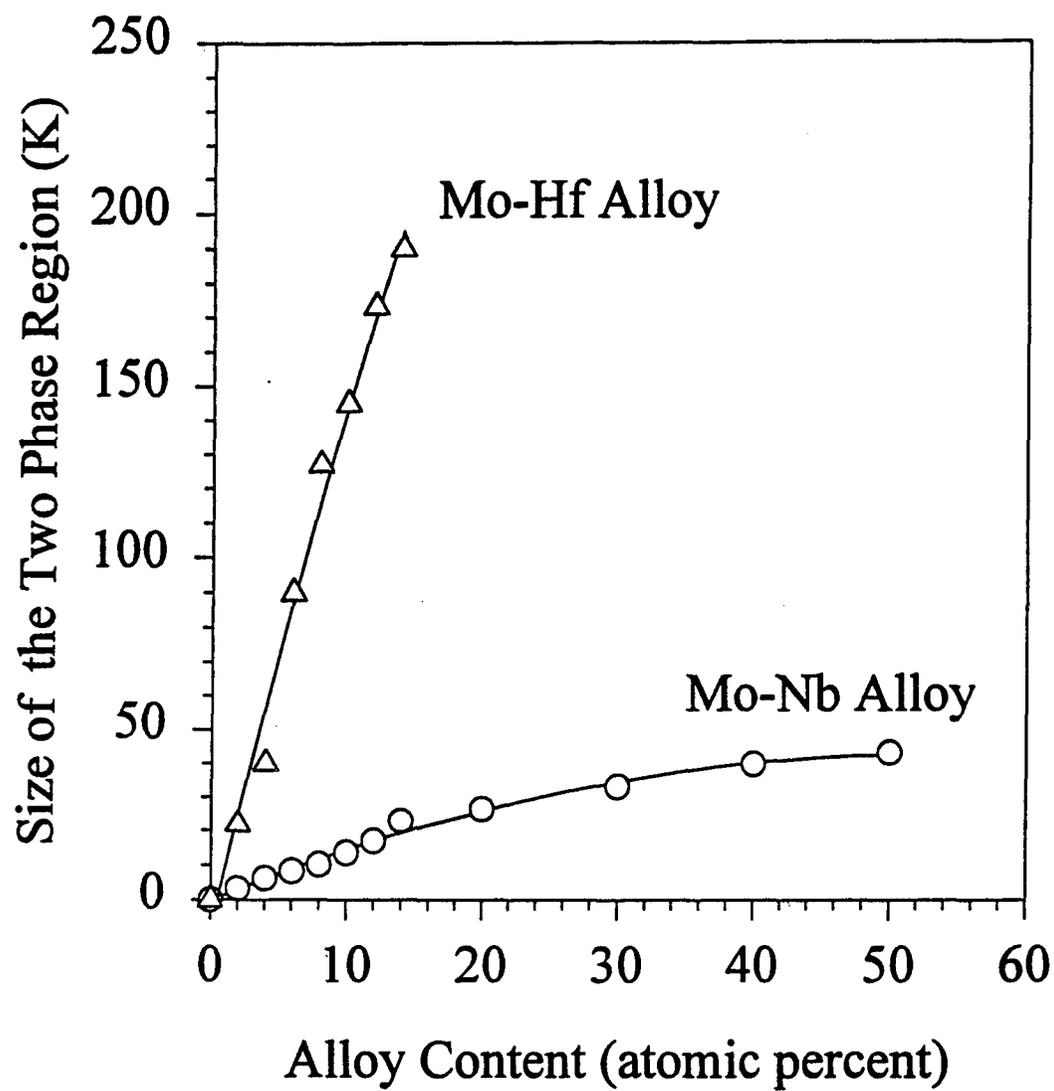
Figure 19. Temperature difference between the liquidus and solidus lines of the Mo-Nb and Mo-Hf systems.
