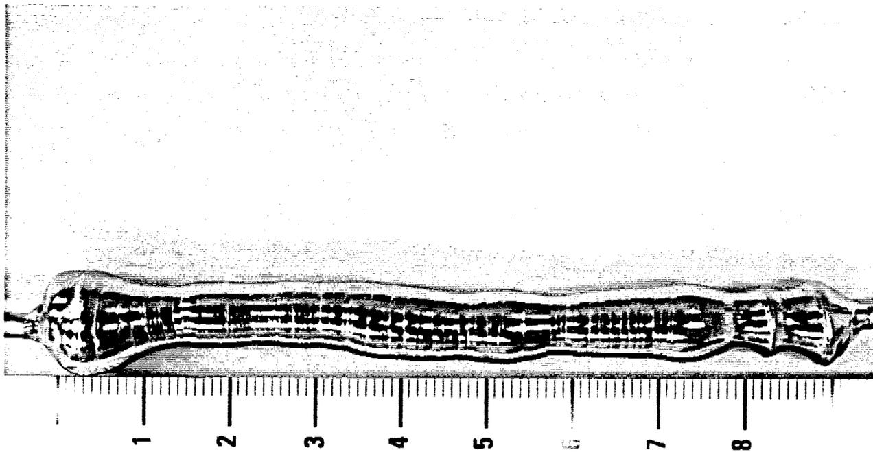
Figure 14. The surface morphology of an as-grown Mo-11%Nb single crystal (scale is centimeter). The smaller rods at the two ends are the support rods.
