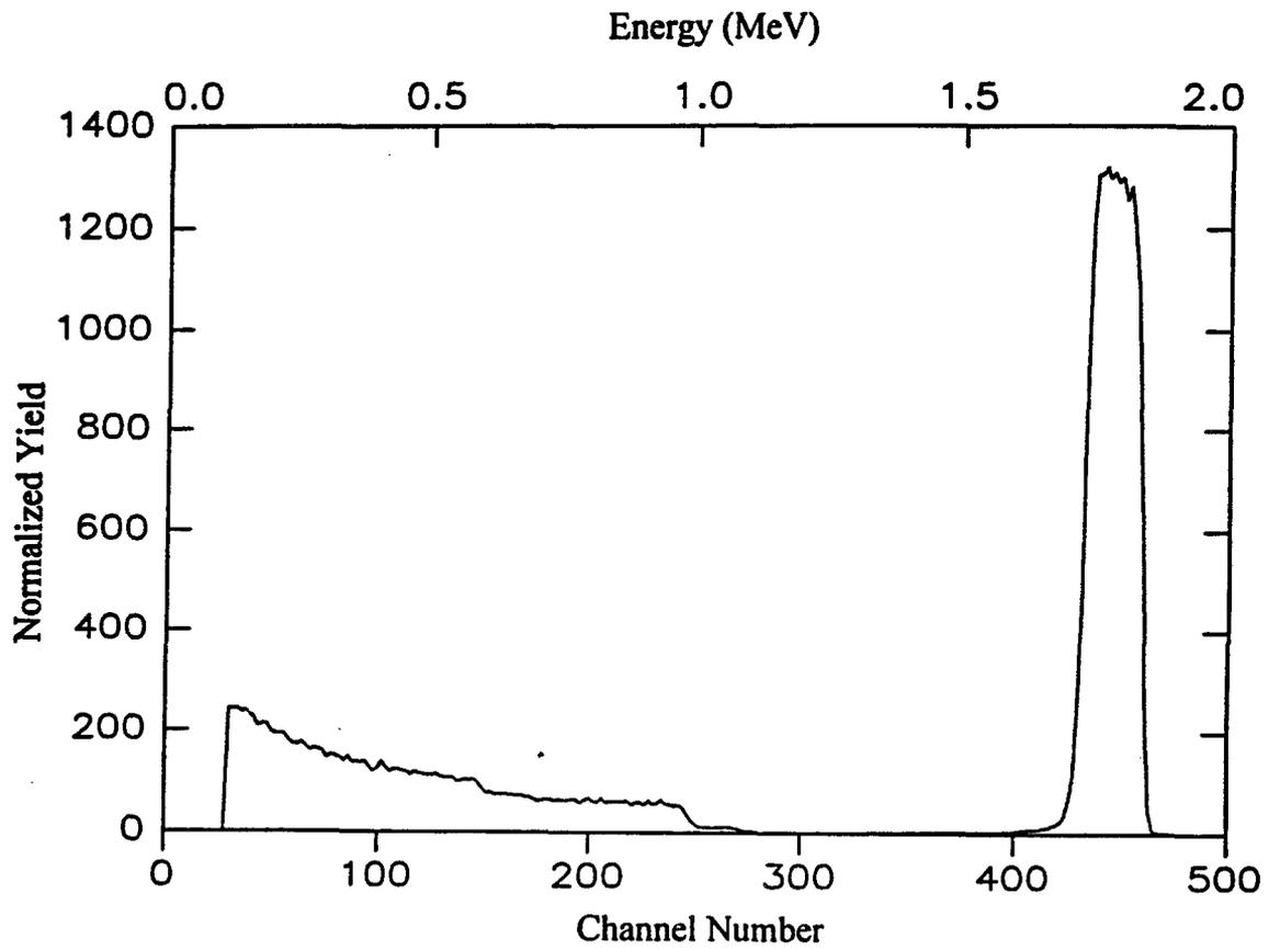
Figure 11. RBS spectrum obtained for sapphire after irradiation of 2 MeV protons at 800 K at an average beam current density of 500 nA/cm<sup>2</sup> for 20 hrs.
