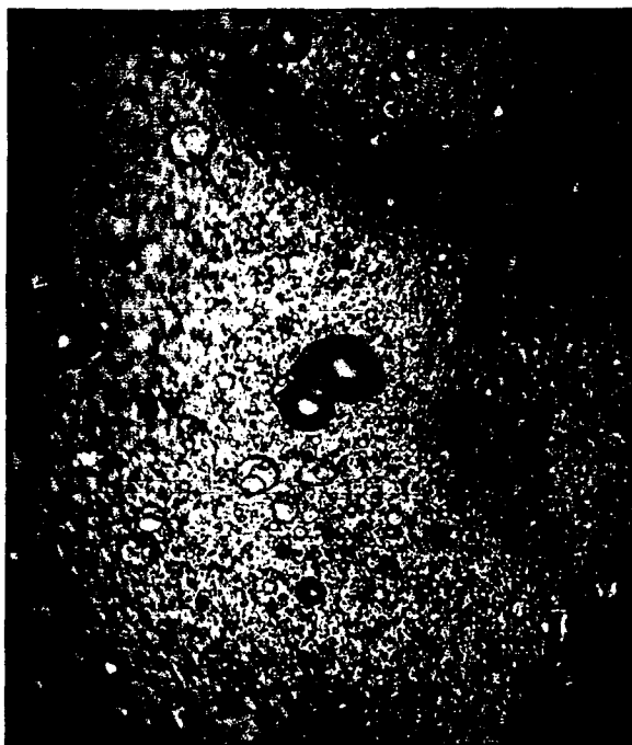
(b) Graphite/Cyanate Ester substrate (200x).
