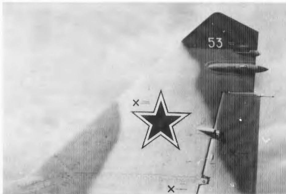
Fig. 31—MiG-29 Vertical Stabilizer with Extended-Chord Rudder. Note Large Exposed Rudder Actuator Hinge and Rear-Hemisphere Threat Warning Antennas
