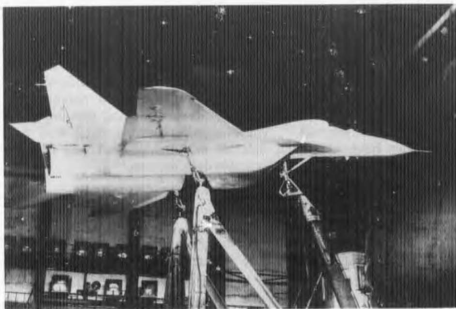
Fig. 34—MiG-29 in Low-Speed Wind Tunnel to Test Nonstandard Trailing-Edge Flap Extension
