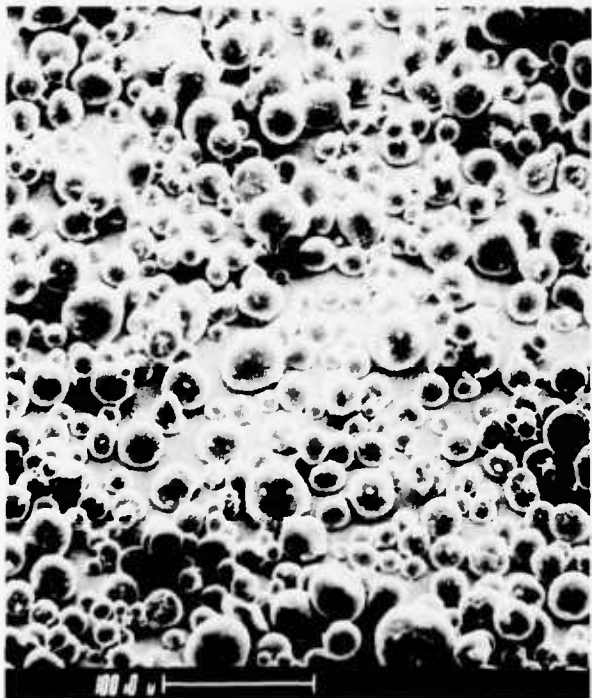
Figure 1. Photomicrographs taken by scanning electron microscopy of microcapsules made with the physiological salt of poly(l-C) and prepared with a DL-PLG excipient: Batches E100-019 and E100-020.
