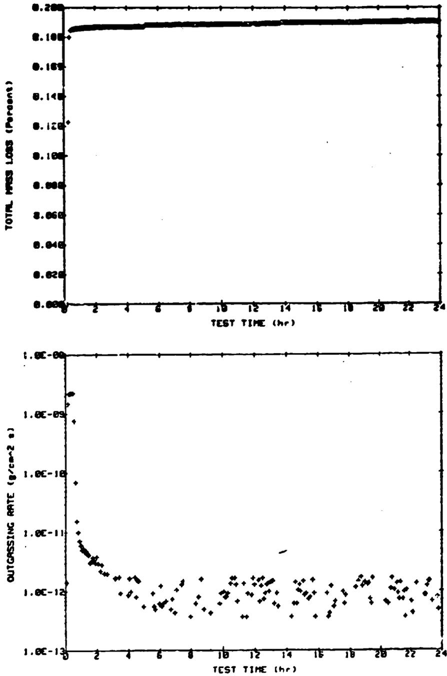
Fig. A-3 Total Mass Loss and Outgassing Rate as Functions of Time for a Kapton Sample at 75°C.
