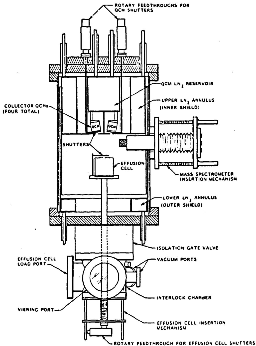
Fig. 3-2 Schematic of the Main Test Chamber
