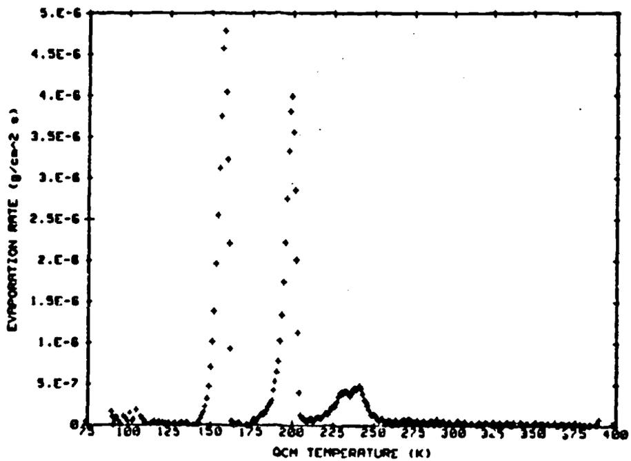
Fig. A-6 QTGA Data for Outgassing Products Collected on the 90 K QCM from an R-2560 Sample at 75°C. Mass of Collected Outgassing Products Remaining on the QCM and Evaporation Rate from the QCM as Functions of Temperature.
