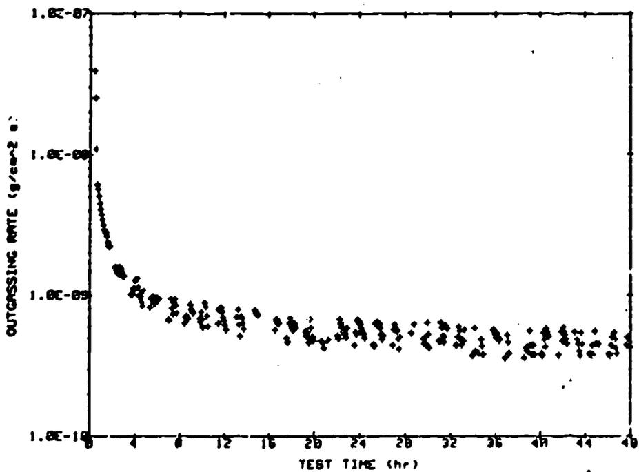
Fig. A-76 Total Mass Loss and Outgassing Rate as Functions of Time for a Krytox 143 AD Sample at 25°C.
