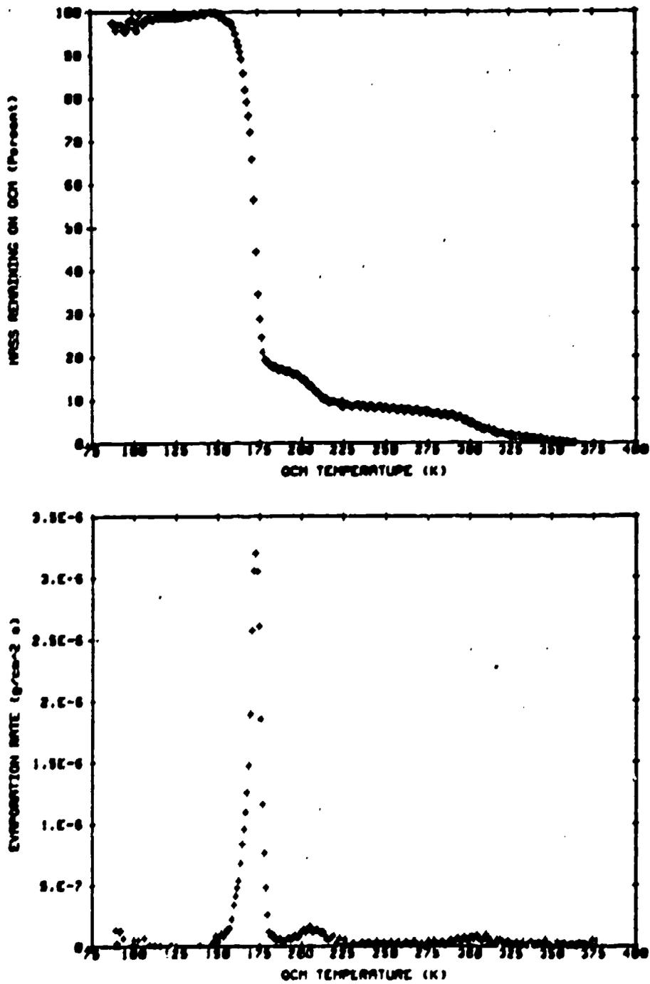
Fig. A-13 QMGA Data for Outgassing Products Collected on the 90 K QCM from an RTV 566 Sample at 75°C. Mass of Collected Outgassing Products Remaining on the QCM and Evaporation Rate from the QCM as Functions of Temperature.
