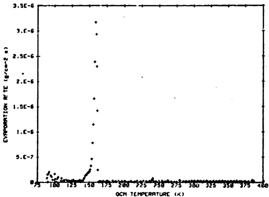
Fig. A-34 QTGA Data for Outgassing Products Collected on the 90 K QCM from a Kapton Sample at 75°C. Mass of Collected Outgassing Products Remaining on the QCM and Evaporation Rate from the QCM as Functions of Temperature.
