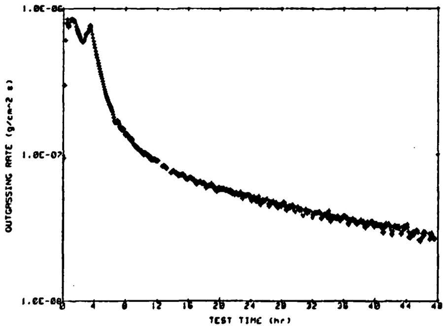
Fig. A-1 Total Mass Loss and Outgassing Rate as Functions of Time for an R-2560 Sample at 125°C.
