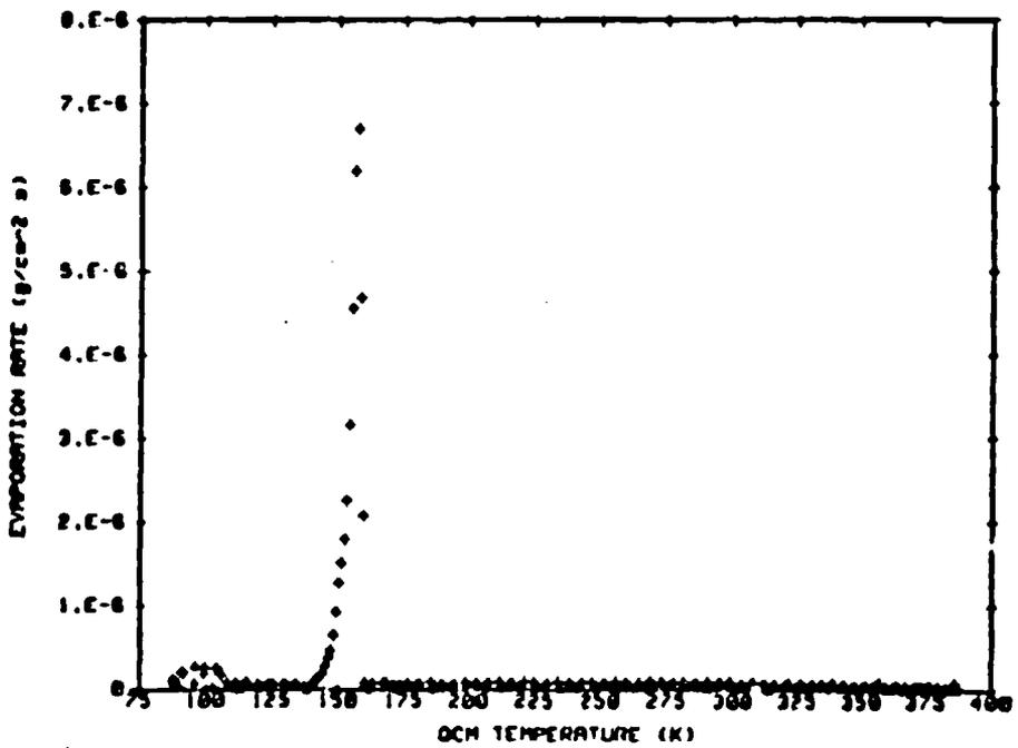
Fig. A-157 QTGA Data for Outgassing Products Collected on the 90 K QCM from an AS4/3501-6 (Source B) Sample at 125°C. Mass of Collected Outgassing Products Remaining on the QCM and Evaporation Rate from the QCM as Functions of Temperature.
