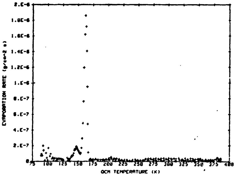
Fig. A-31 QTGA Data for Outgassing Products Collected on the 90 K QCM from a Kapton Sample at 125°C. Mass of Collected Outgassing Products Remaining on the QCM and Evaporation Rate from the QCM as Functions of Temperature.
