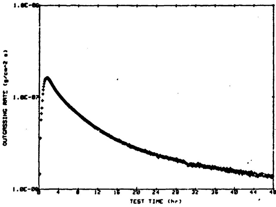
Fig. A-22 Total Mass Loss and Outgassing Rate as Functions of Time for a DC 6-1104 Sample at 125°C.
