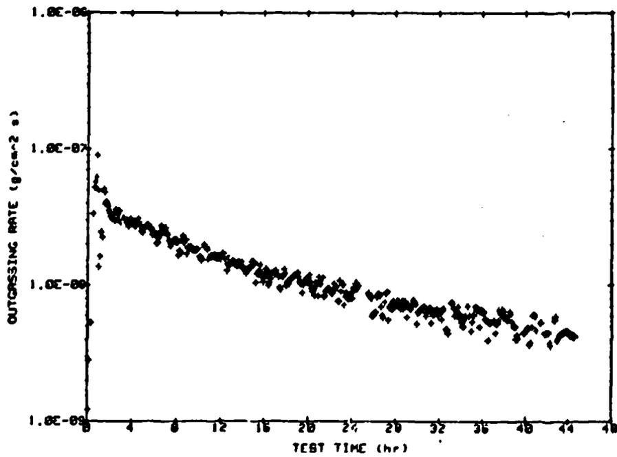
Fig. A-73 Total Mass Loss and Outgassing Rate as Functions of Time for a Krytox 143 AD Sample at 75°C.
