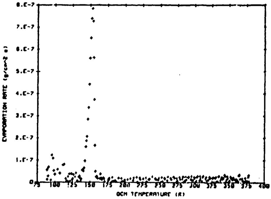
Fig. A-136 Q/GA Data for Outgassing Products Collected on the 90 K QCM from an AS4/PEEK Sample at 125°C. Mass of Collected Outgassing Products Remaining on the QCM and Evaporation Rate from the QCM as Functions of Temperature.
