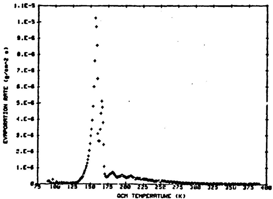
Fig. A-24 QTGA Data for Outgassing Products Collected on the 90 K QCM from a DC 6-1104 Sample at 125°C. Mass of Collected Outgassing Products Remaining on the QCM and Evaporation Rate from the QCM as Functions of Temperature.
