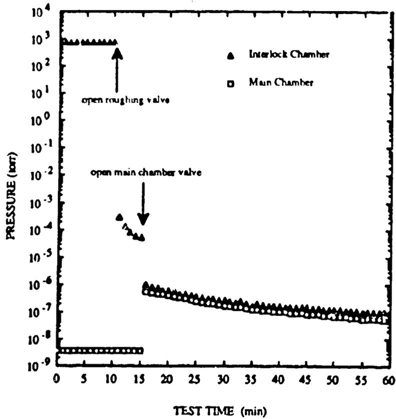
Fig. 3-4 Main and Interlock Chamber Pressures during Effusion Cell Insertion.
