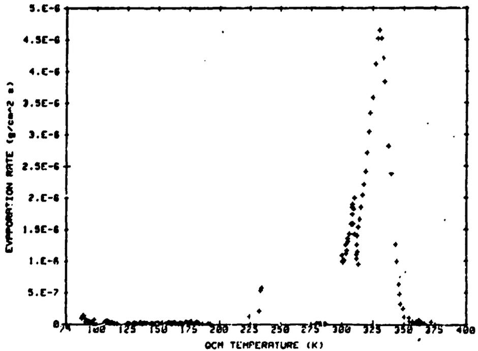
Fig. A-72 QTGA Data for Outgassing Products Collected on the 90 K QCM from a Krytox 143 AD Sample at 125°C. Mass of Collected Outgassing Products Remaining on the QCM and Evaporation Rate from the QCM as Functions of Temperature.
