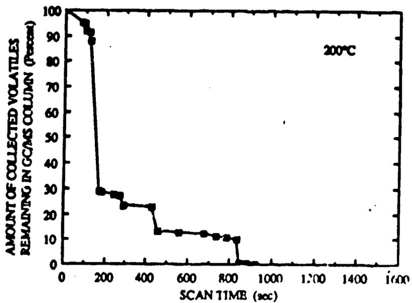
Fig. A-28 Amount of Collected Volatiles Remaining in GC/MS Column from DC 6-1104 at 125°C and 200°C
