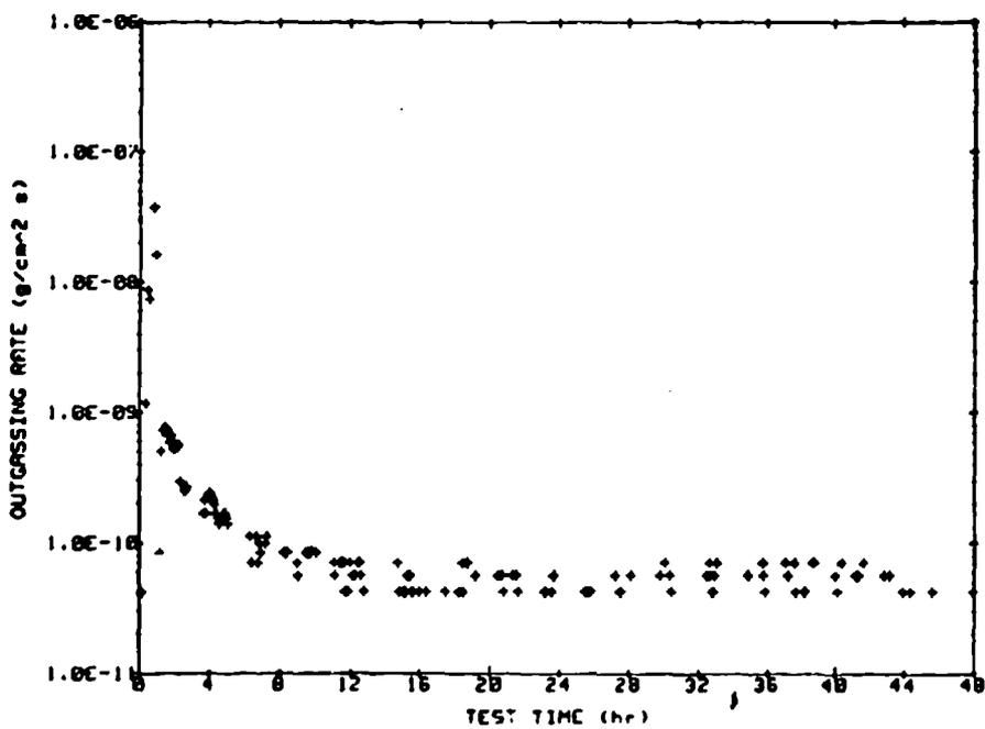
Fig. A-53 Total Mass Loss and Outgassing Rate as Functions of Time for a Brayco 815Z Sample at 75°C.
