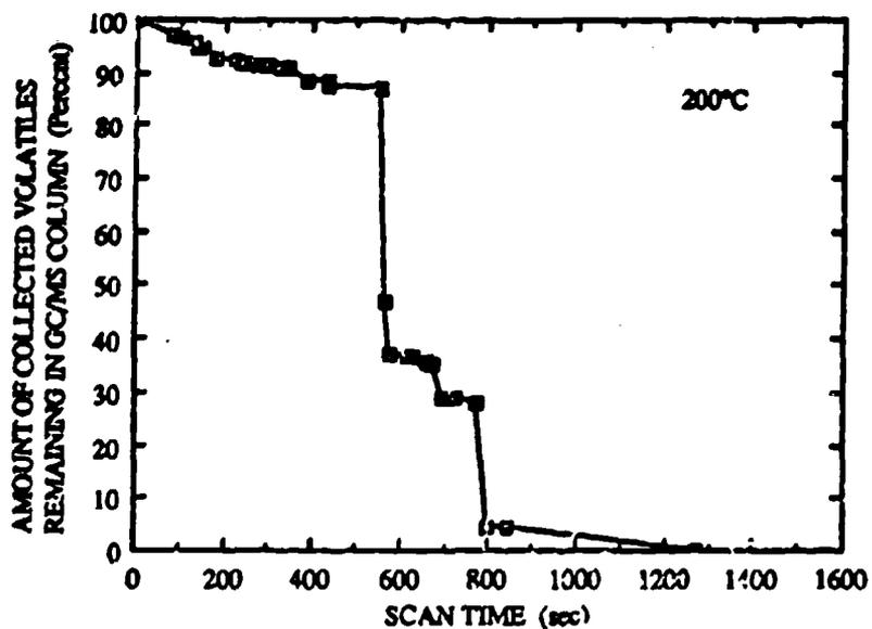
Fig. A-103 Amount of Collected Volatiles Remaining in GC/MS Column from Chemglaze Z306 at 125°C and 200°C
