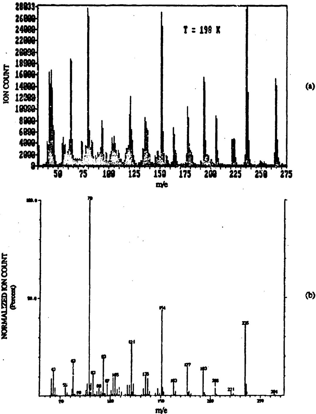
Fig. 5-38 Comparison of Mass Spectra Obtained During QTA/MS of the Outgassing Products from R-2560 at 125°C and GC/MS of the R-2560 at 200°C. (a) QTA/MS Mass Spectrum of Evaporating Flux at a QCM Temperature of 198 K and (b) GC/MS Mass Spectrum for Alkyl Silicate at Scan = 596 s.
