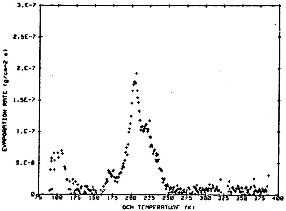
Fig. A-109 QTGA Data for Outgassing Products Collected on the 90 K QCM from a DC Q9-6313 Sample at 75°C. Mass of Collected Outgassing Products Remaining on the QCM and Evaporation Rate from the QCM as Functions of Temperature.
