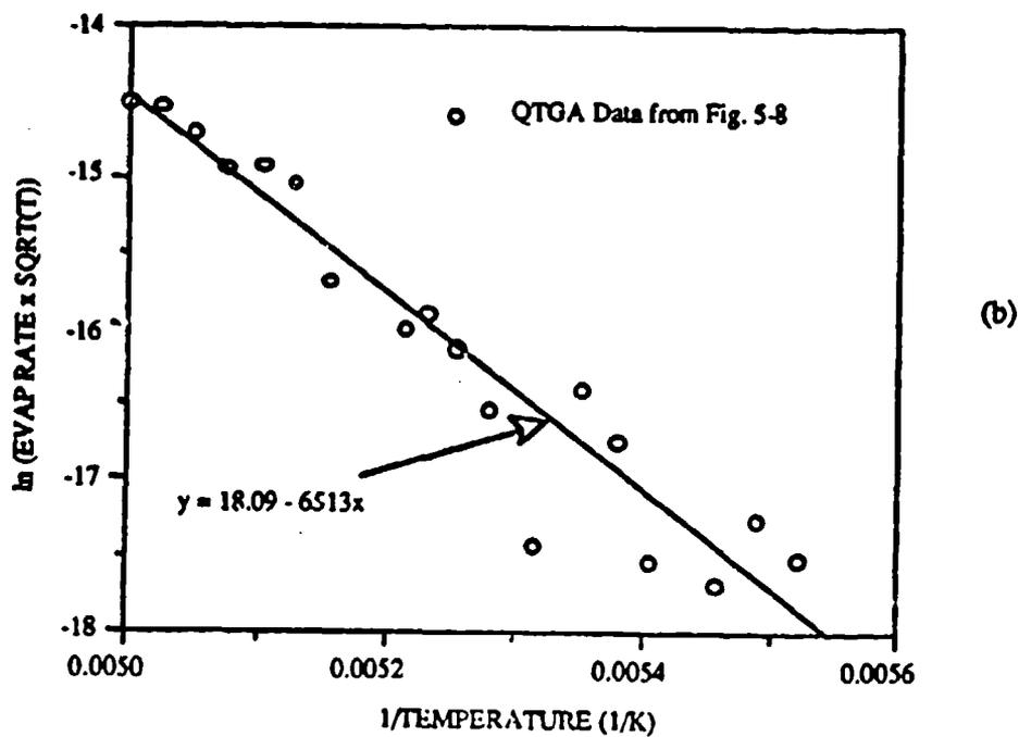
Fig. 5-9 Evaporation Rate Plots ( $m_e \sqrt{T}$  versus  $1/T$ ) of the 158 K and 198 K Species:
