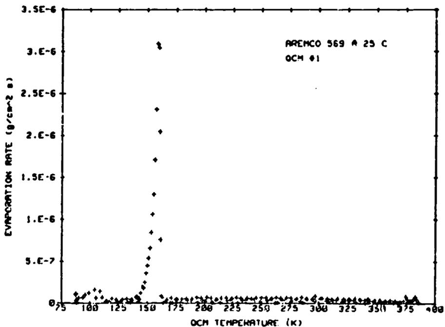
Fig. A-122 QTGA Data for Outgassing Products Collected on the 90 % QCM from an Aremco 569 Sample at 25°C Mass of Collected Outgassing Products Remaining on the QCM and Evaporation Rate from the QCM as Functions of Temperature.
