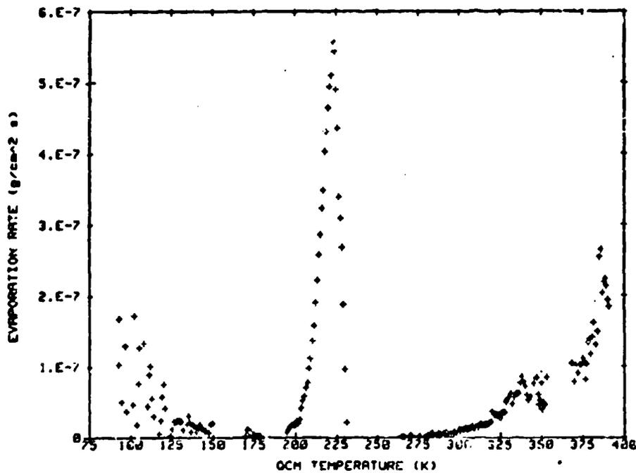
Fig. A-58 QTGA Data for Outgassing Products Collected on the 90 K QCM from a Brayco 815Z Sample at 100°C. Mass of Collected Outgassing Products Remaining on the QCM and Evaporation Rate from the QCM as Functions of Temperature.
