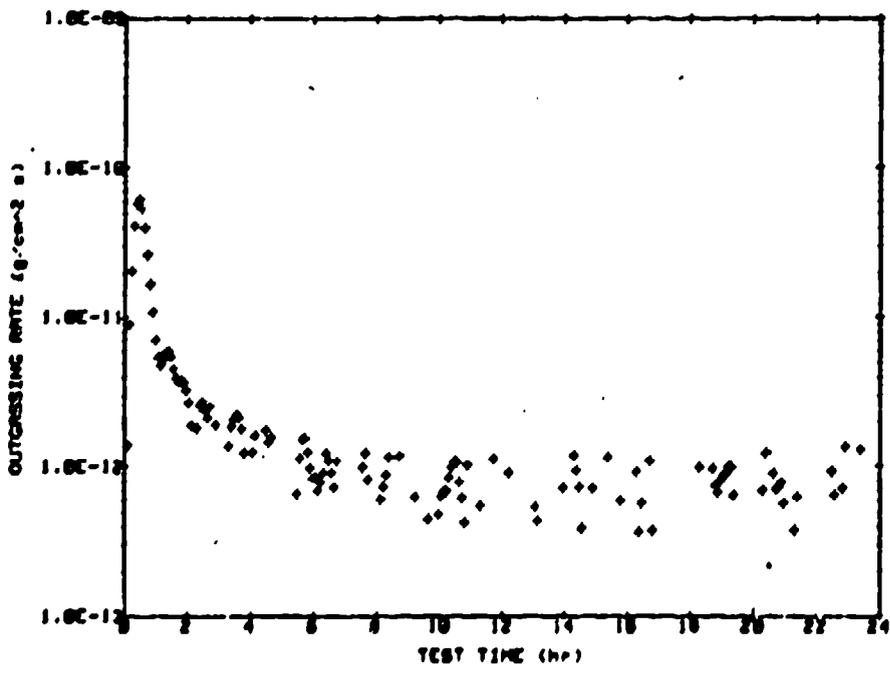
Fig. A-43 Total Mass Loss and Outgassing Rate as Functions of Time for an FEP Teflon Sample at 125°C.
