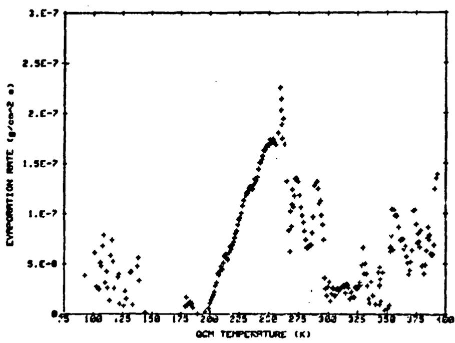
Fig. A-65 QTGA Data for Outgassing Products Collected on the 90 K QCM from a Braycote 600 Sample at 75°C. Mass of Collected Outgassing Products Remaining on the QCM and Evaporation Rate from the QCM as Functions of Temperature.
