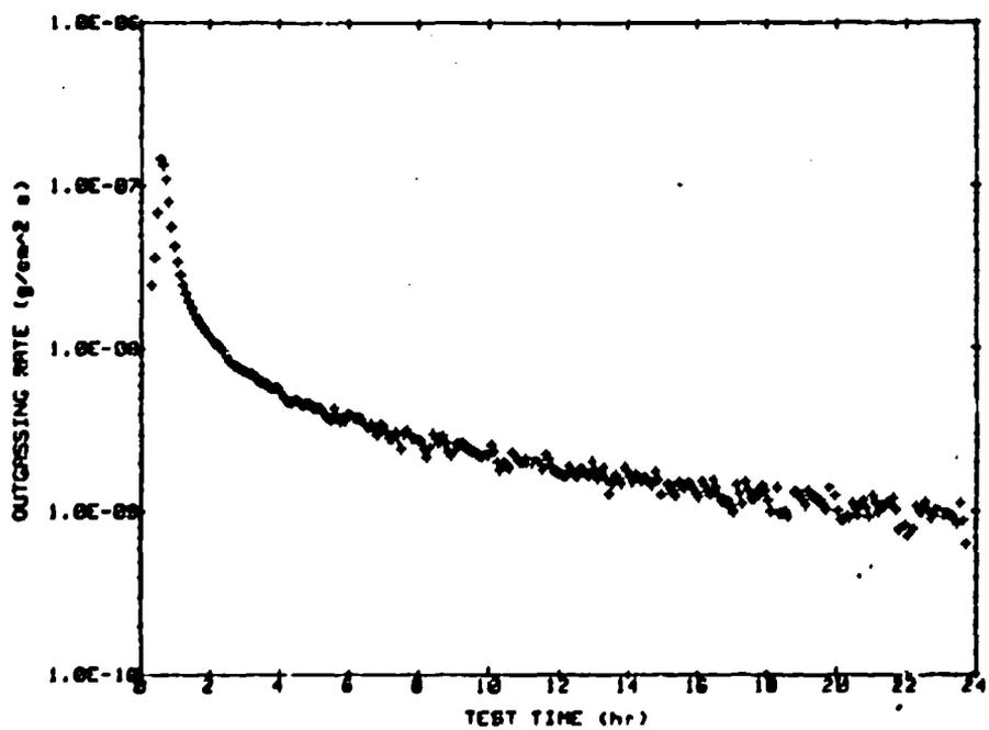
Fig. A-90 Total Mass Loss and Outgassing Rate as Functions of Time for an S/13G/LO-V10 Sample at 125°C.
