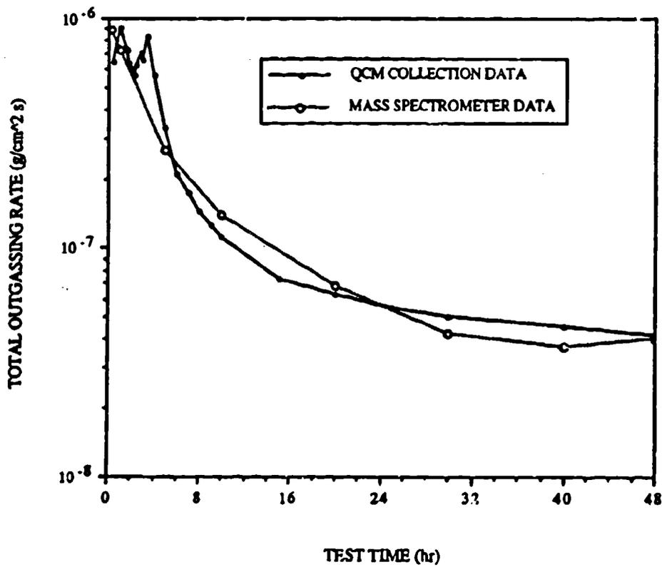
Fig. 5-46 Comparison of the Total Outgassing Rate Measured by QCM Collection and Calculated from Mass Spectrometer Ion Count Data for R-2560 at 125°C.
