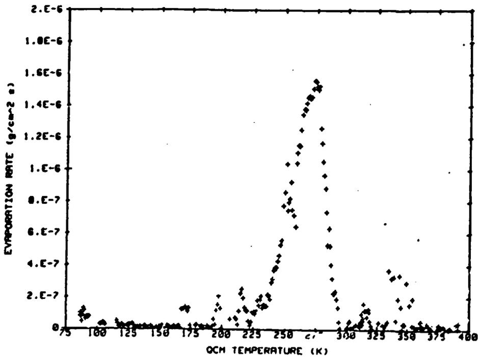
Fig. A-75 QTGA. Data for Outgassing Products Collected on the 90 K QCM from a Krytox 143 AD Sample at 75°C. Mass of Collected Outgassing Products Remaining on the QCM and Evaporation Rate from the QCM as Function of Temperature.
