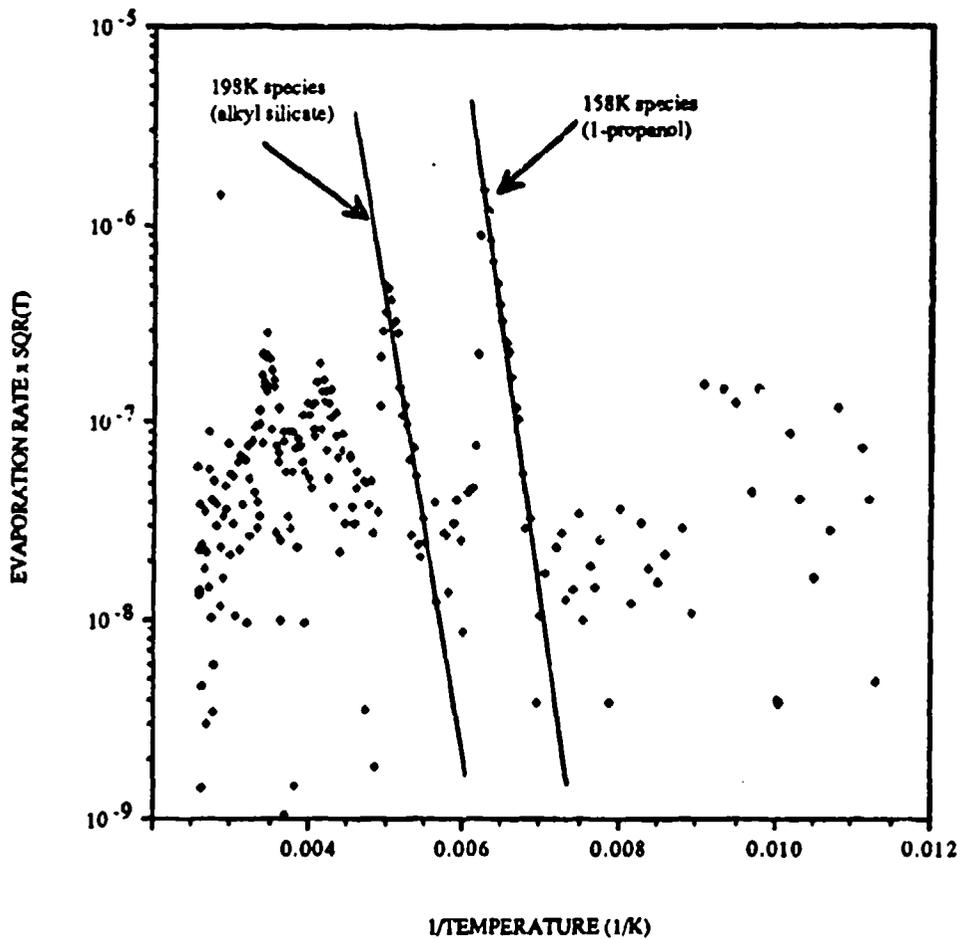
Fig. 5-8 Differential QCM Thermogravimetry Data for Outgassing Products Collected on the 90 K QCM from R-2560 at 125°C ( $\ln_q \sqrt{T}$  versus  $1/T$ ).
