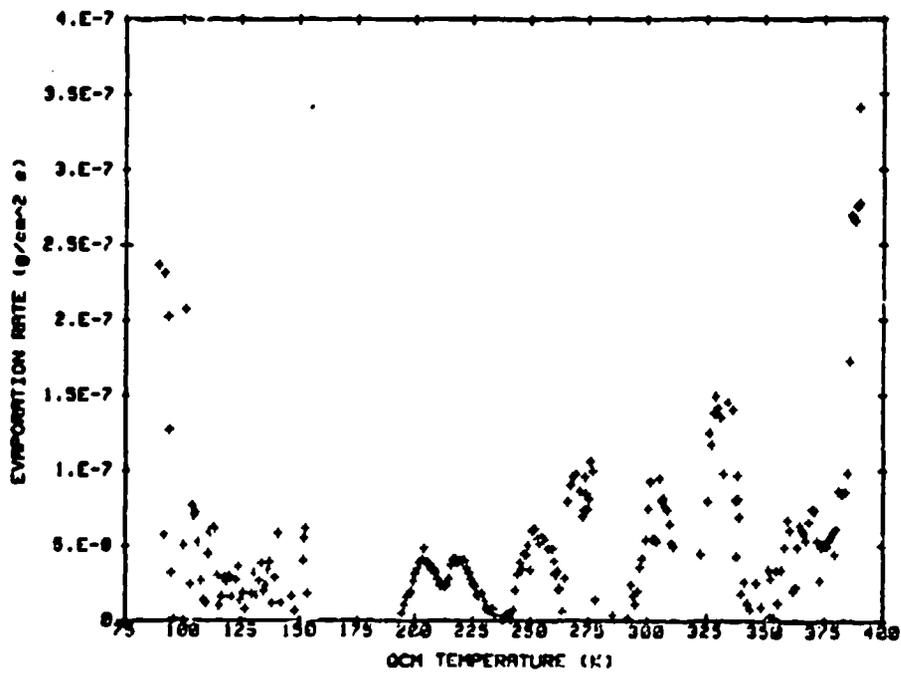
Fig. A-52 QTGA Data for Outgassing Products Collected on the 90 K QCM from a Brayco 815Z Sample at 125°C. Mass of Collected Outgassing Products Remaining on the QCM and Evaporation Rate from the QCM as Functions of Temperature.
