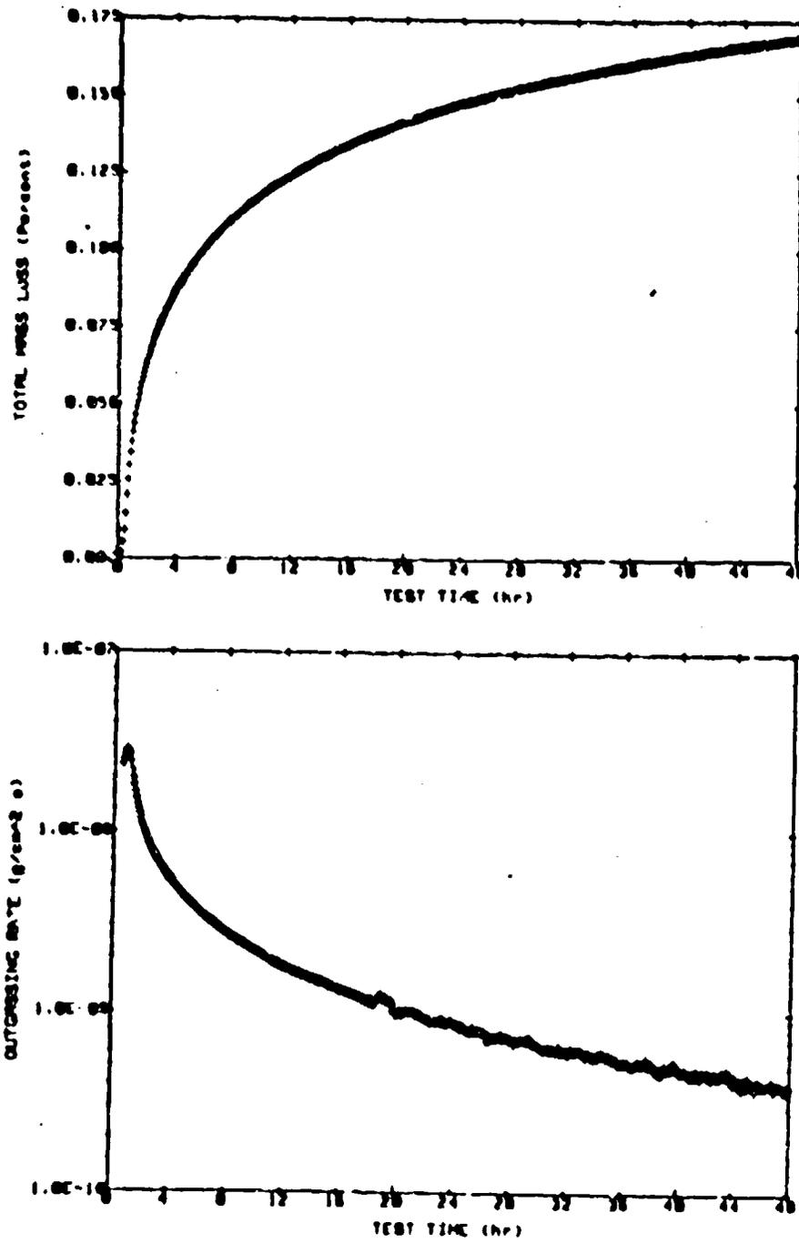
Fig. A-148 Total Mass Loss and Outgassing Rate as Functions of Time for an AS4/3501-6 (Source *L*.) Sample at 125°C.
