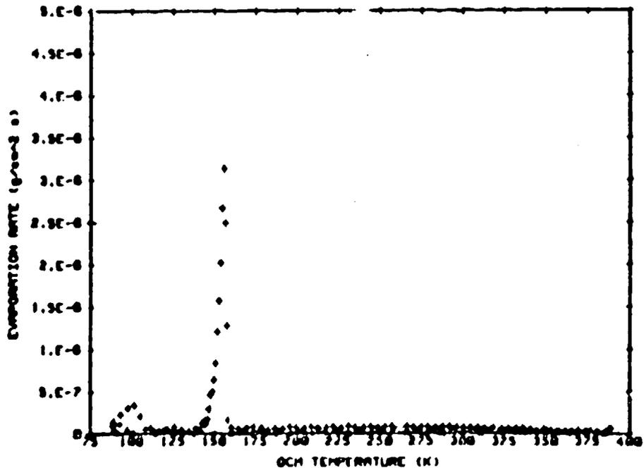
Fig. A-160 QTGA Data for Outgassing Products Collected on the 90 K QCM from an AS4/3501-6 (Source B) Sample at 75°C. Mass of Collected Outgassing Products Remaining on the QCM and Evaporation Rate from the QCM as Functions of Temperature.
