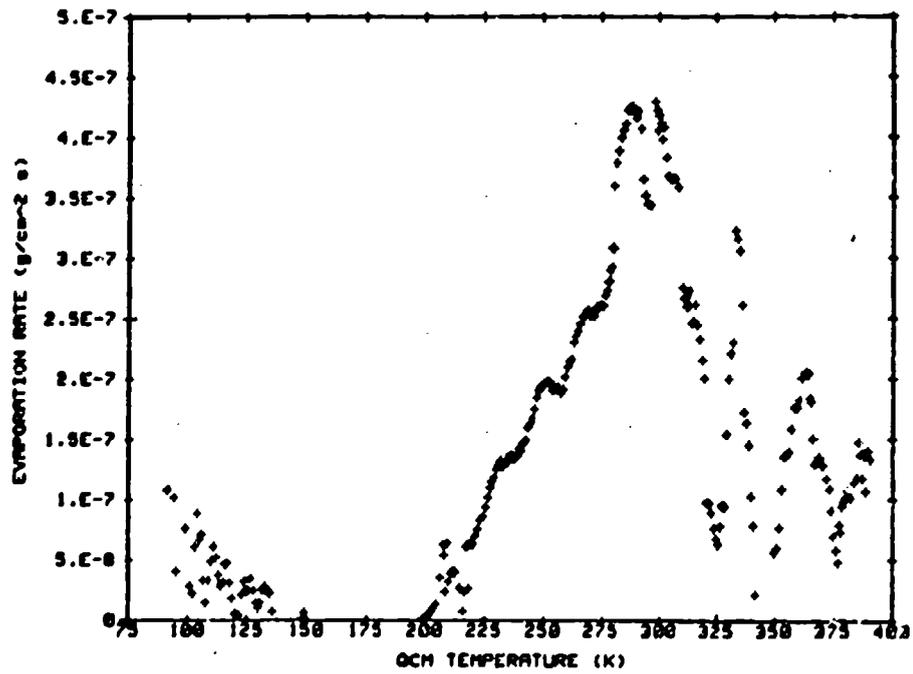
Fig. A-62 QTGA Data for Outgassing Products Collected on the 90 K QCM from a Braycote 600 Sample at 125°C. Mass of Collected Outgassing Products Remaining on the QCM and Evaporation Rate from the QCM as Functions of Temperature.
