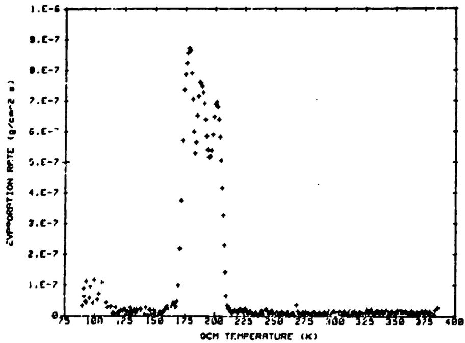
Fig. A-102 QTGA Data for Outgassing Products Collected on the 90 K QCM from a Chemglaze Z306 Sample at 75°C. Mass of Collected Outgassing Products Remaining on the QCM and Evaporation Rate from the QCM as Functions of Temperature.
