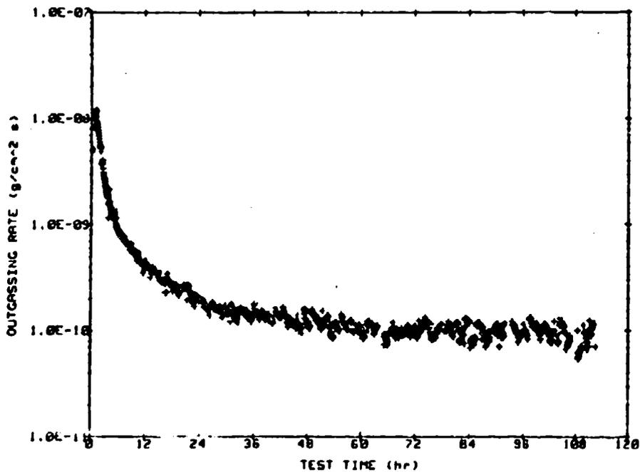
Fig. A-107 Total Mass Loss and Outgassing Rate as Functions of Time for a DC Q9-6313 Sample at 75°C.
