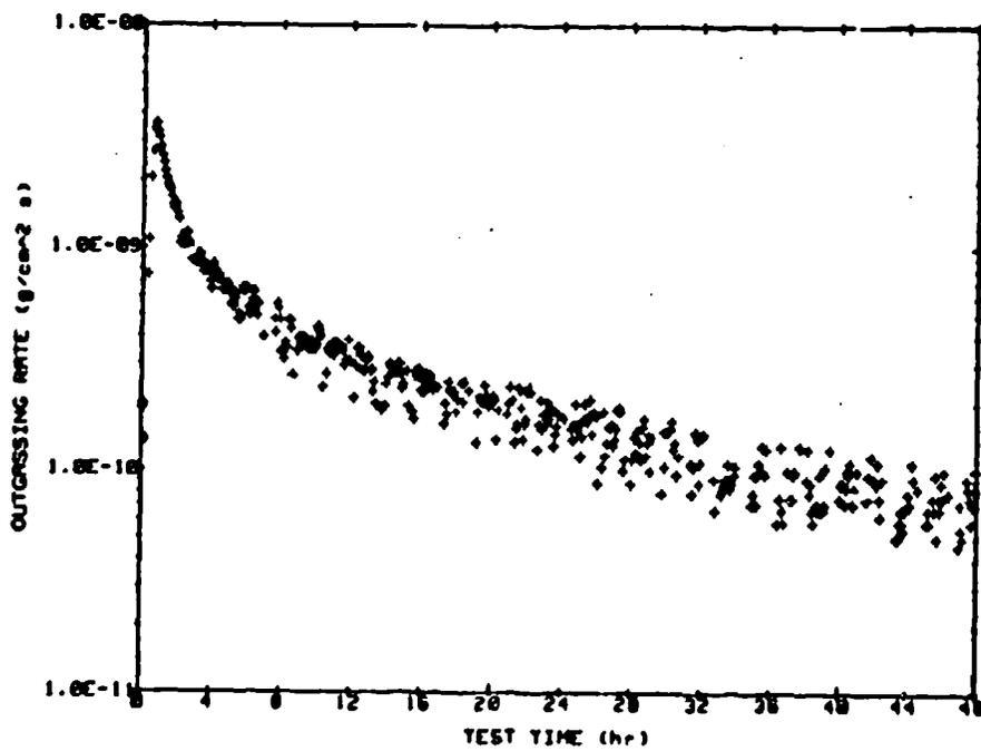
Fig. A-134 Total Mass Loss and Outgassing Rate as Functions of Time for an AS4/PEEK Sample at 125°C.
