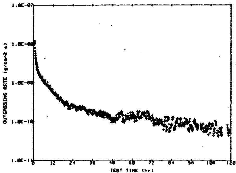
Fig. A-110 Total Mass Loss and Outgassing Rate as Functions of Time for a DC Q9-6313 Sample at 25°C.
