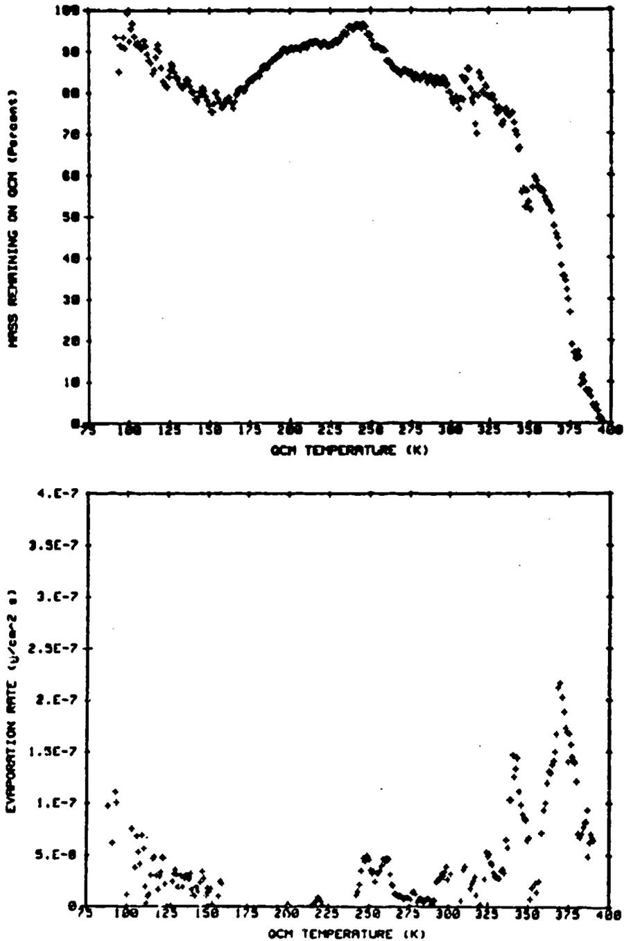
Fig. A-55 QMGA Data for Outgassing Products Collected on the 90 K QCM from a Brayco 815Z Sample at 75°C. Mass of Collected Outgassing Products Remaining on the QCM and Evaporation Rate from the QCM as Functions of Temperature.
