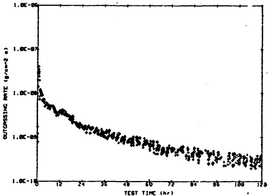
Fig. A-63 Total Mass Loss and Outgassing Rate as Functions of Time for a Braycote 600 Sample at 75°C.
