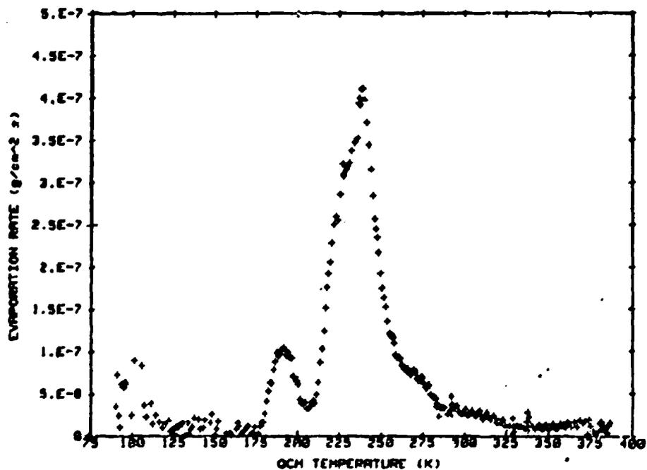
Fig. A-85 QTGA Data for Outgassing Products Collected on the 90 K QCM from a VacKote MLD 73-91 Sample at 75°C. Mass of Collected Outgassing Products Remaining on the QCM and Evaporation Rate from the QCM as Functions of Temperature.
