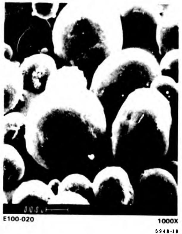
Figure 4. Photomicrographs taken by scanning electron microscopy of prototype poly(l-C) microcapsules prepared with a DL-PLG excipient: Batches E100-019 and E100-020.
