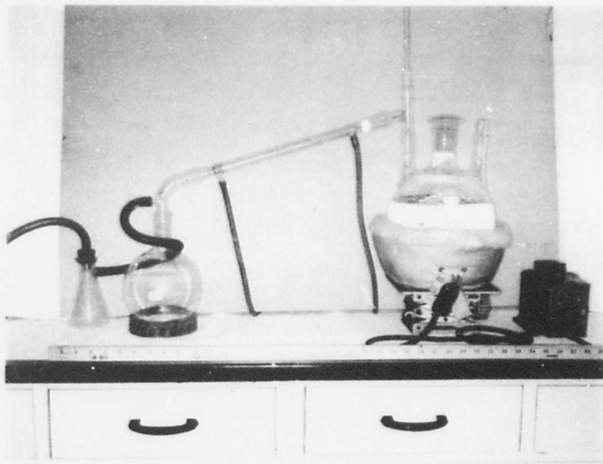
Figure 1. Removal of excess water from glycolic acid.
