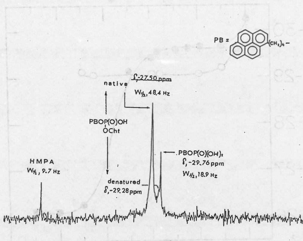
**Fig. 1:**  $^{31}\text{P}$ -nmr spectra of the aged conjugate, pyrenebutyl-O-P(O)(OH)Cht, (1 mM, pH 4.1). Chemical shifts were assigned to HMPA. The diacid signal stems from the corresponding dichloro inhibitor that was not removed completely after the inhibition.
