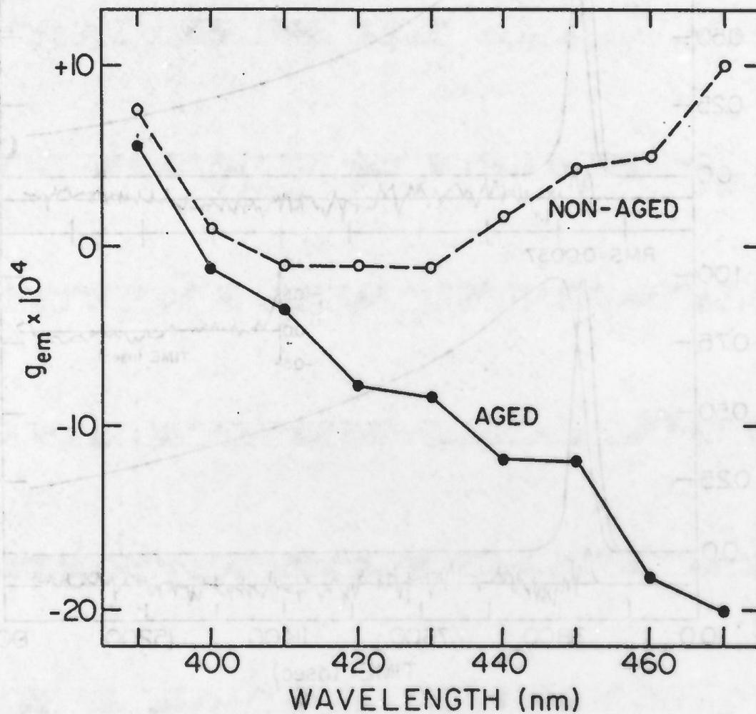
**Fig. 6:** Circularly polarized luminescence (CPL) spectra of aged [pyrenebutyl-O-P(O)(OH)Cht] and non-aged [pyrenebutyl-O-P(O)(OC<sub>2</sub>H<sub>5</sub>)Cht] conjugates of chymotrypsin. The curves show the emission anisotropy factor,  $g_{em}$ , as a function of wavelength for the aged (●—●) and non-aged (○----○) conjugates.
