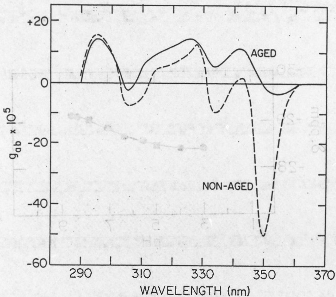
**Fig. 4:** Circular dichroism (CD) spectra of aged [pyrenebutyl-O-P(O)(OH)Cht] and non-aged [pyrenebutyl-O-P(O)(OC<sub>2</sub>H<sub>5</sub>)Cht] conjugates of chymotrypsin. The curves display the absorption anisotropy factor,  $g_{ab}$ , as a function of wavelength for the aged (—) and non-aged (---) conjugates.
