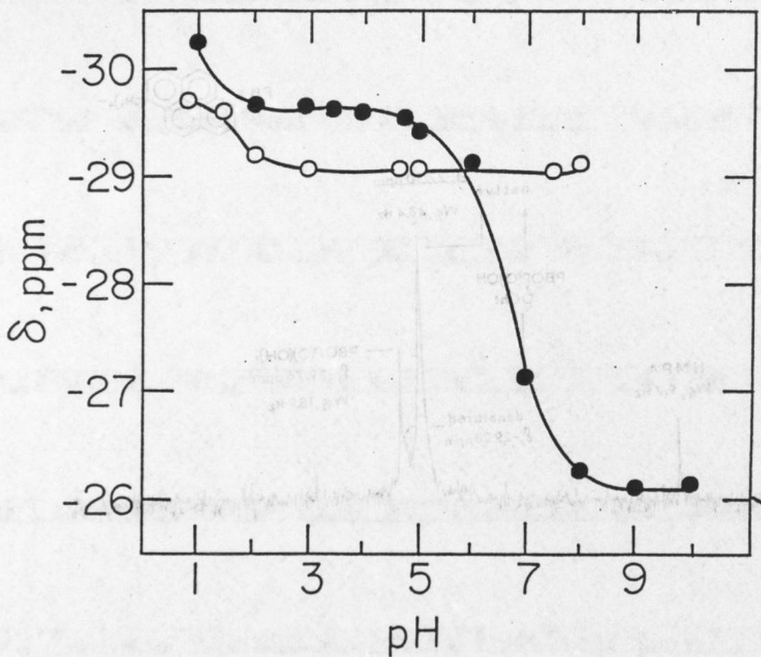
Fig. 2: pH chemical shift profile for mono- and diacid phosphates.  $\delta$  is related to HMPA. ○—○,  $(C_2H_5O)_2P(O)OH$ ; ●—●,  $(C_2H_5O)P(O)(OH)_2$ .
