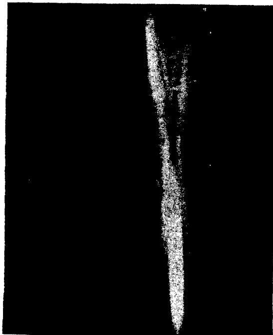
Figure 21 Lens Focused Sound Beam of Linear Array Transducer
