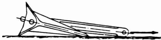
Anchor dragging on hard seafloor with fluke tips unable to bite in.
