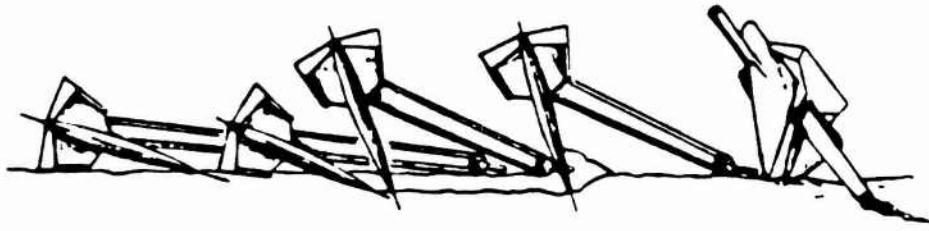
Anchor standing up but tipping to side and dragging.
