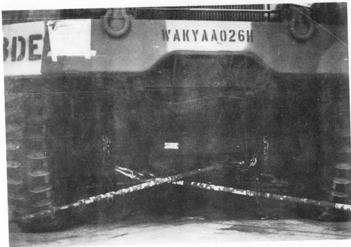
Figure 5-4. Lashings applied over axles on USNS Meteor .
