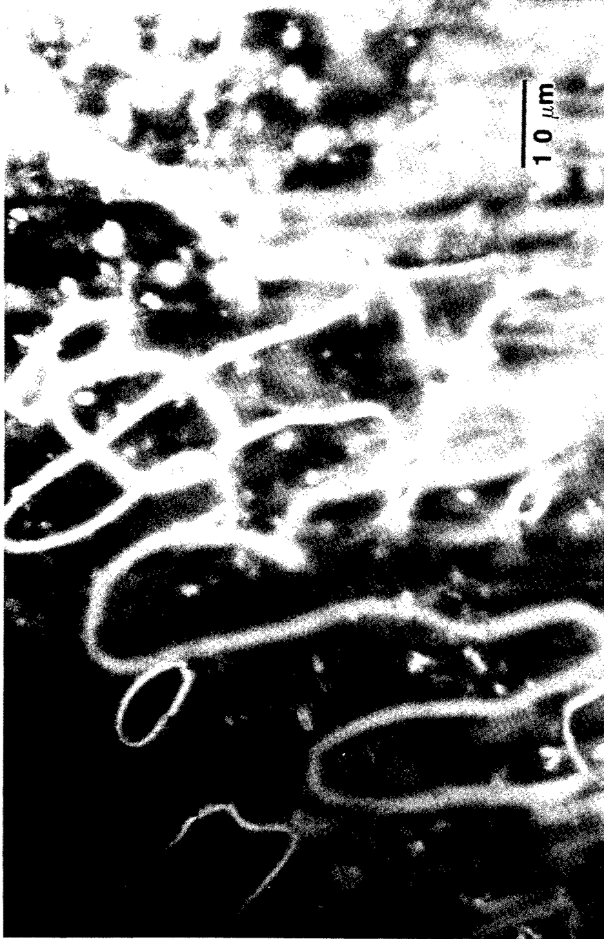
Figure 3.6: Schlieren texture in 9% PBT in MSA after 48 hours relaxation
