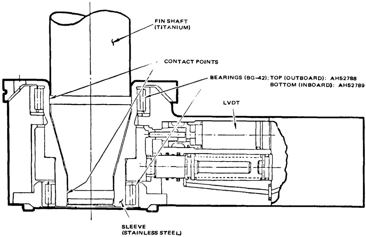
Figure 1. ASALM – Activator design-bearing detail (MDAC).
