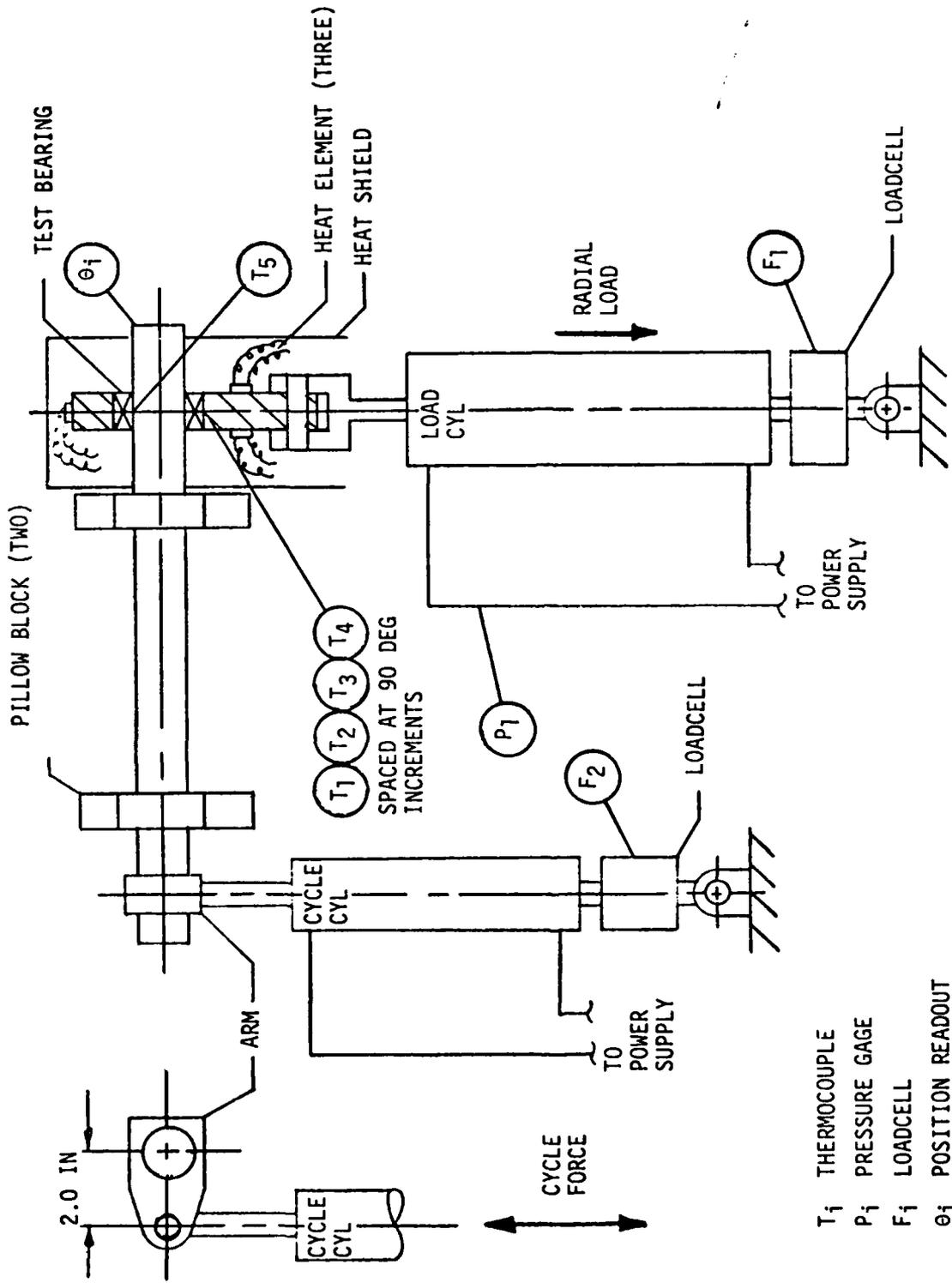
Figure 1-1. Bearing/Lubrication Test Set-up Schematic
