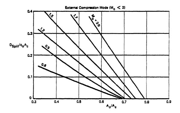
Figure 31. Performance Characteristics for Inlet Configuration #14 (continued)
