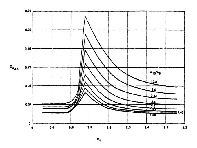
Figure 43. Drag for a Single Round C-D Nozzle Installation
