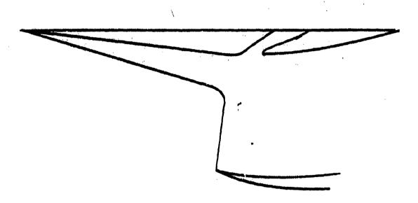
Figure 16. Fixed-Geometry Two-Shock Inlet Design for Mach 1.60
