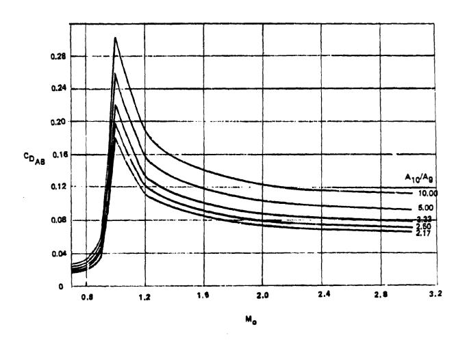
Figure 49. Drag for a Twin-Round Plug Nozzle Installation
