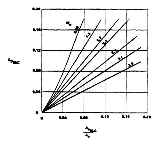
Figure 33. Performance Characteristics for Inlet Configuration #15 (continued)
