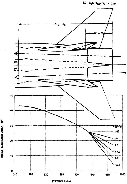
Figure 56. Nozzle/Aftbody Area Distribution for a Twin 2-D Wedge Nozzle Installation 175
