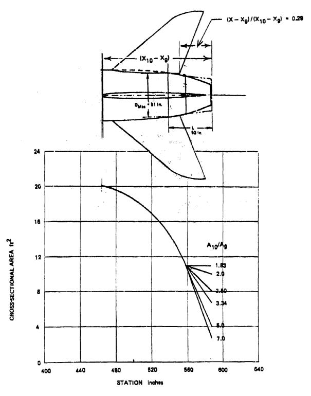
Figure 42. Nozzle/Aftbody Area Distribution for a Single Round C-D Nozzle Installation
