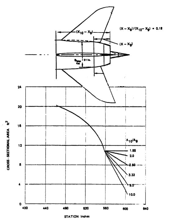
Figure 46. Nozzle/Aftbody Area Distribution for a Single Round Plug Nozzle Installation
