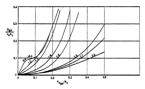
Figure 31. Performance Characteristics for Inlet Configuration #14 (continued)
