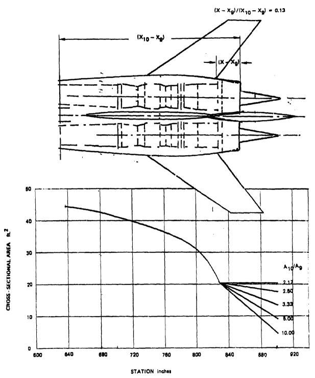
Figure 48. Nozzle/Aftbody area Distribution for a Twin Round Plug Nozzle
