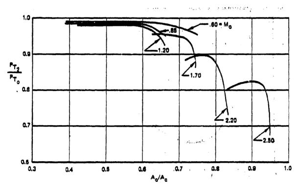
Figure 21. Performance Characteristics for Inlet Configuration #9
