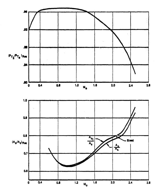
Figure 21. Performance Characteristics for Inlet Configuration #9 (continued)
