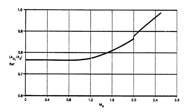
Figure 29. Performance Characteristics for Inlet Configuration #13 (continued)
