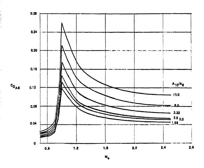
Figure 47. Drag for a Single Round Plug Nozzle Installation
