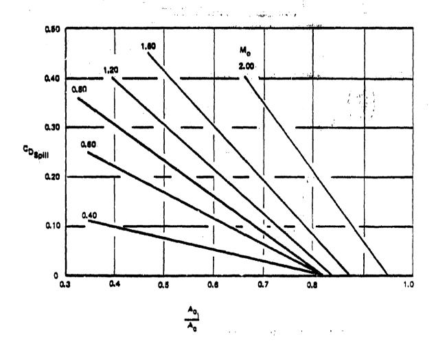
Figure 17. Performance Characteristics for Inlet Configuration #7 (continued)
