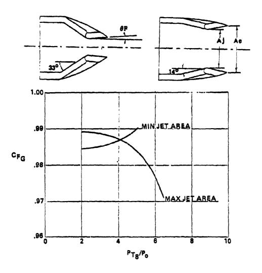
Figure 60 Gross Thrust Coefficient for a 2-D/C-D Nozzle
