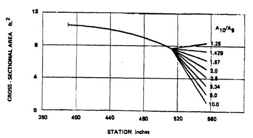
Figure 54. Nozzle Aftbody Area Distributon for a Single 2-D Wedge Nozzle Installation
