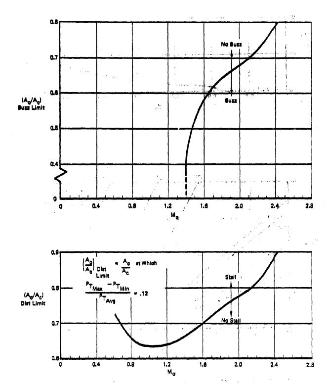
Figure 21. Performance Characteristics for Inlet Configuration #9 (continued)
