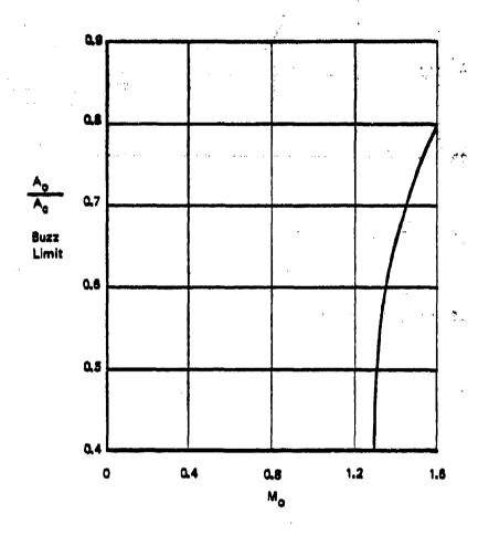
Figure 23. Performance Characteristics for Inlet Configuration #10 (continued)
