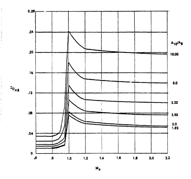
Figure 53. Drag for a Twin 2-D C-D Nozzle Installation
