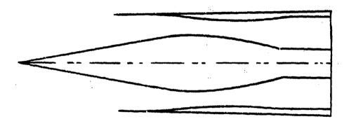
Figure 34. Mach 2.35 Mixed-Compression Axisymmetric Inlet
