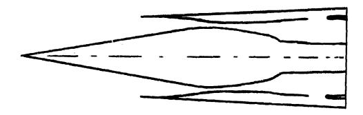
Figure 38. Mach 3.5 Axisymmetric Mixed-Compression Inlet
