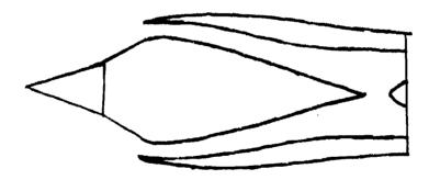
Figure 26. Half-Round External-Compression Inlet for Mach 2.5
