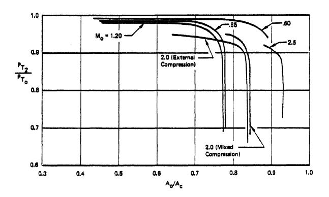
Figure 29. Performance Characteristics for Inlet Configuration #13
