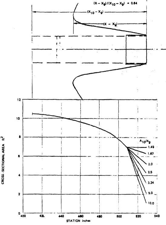
Figure 50. Nozzle/Aftbody Area Distribution for a Single 2-D C-D Nozzle Installation
