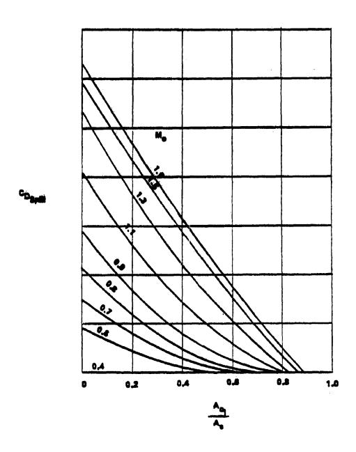
Figure 7. Performance Characteristics for Inlet Configuration #2 (continued)  $^{-\alpha}$
