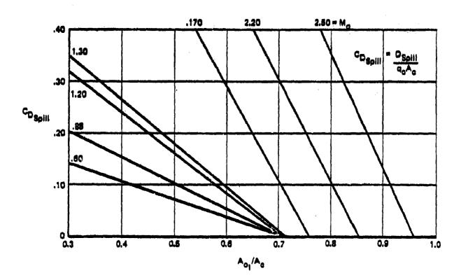
Figure 21. Performance Characteristics for Inlet Configuration #9 (continued)
