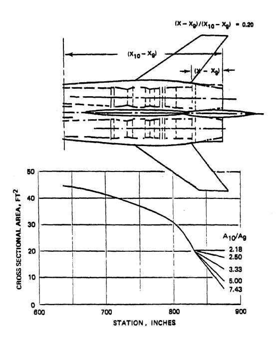
Figure 44 Nozzle/Aftbody Area Distribution for a Twin Round Nozzle Configuration
