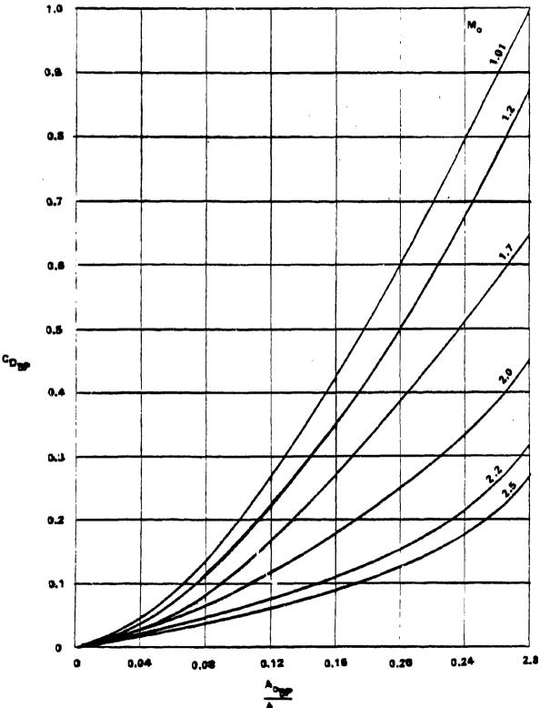
Figure 27. Performance Characteristics for Inlet Configuration #12 (continued) 93
