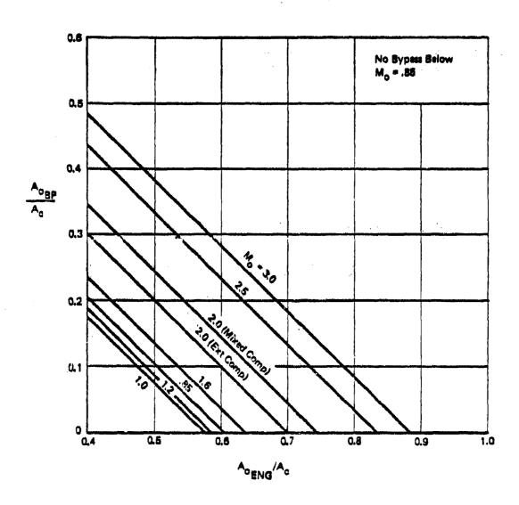
Figure 31. Performance Characteristics for Inlet Configuration #14 (concluded)
