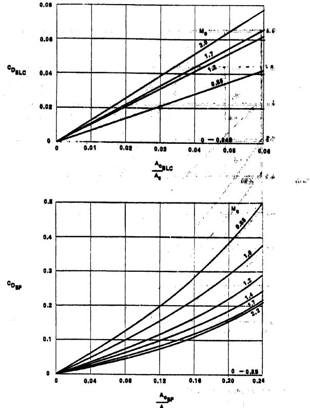
Figure 19. Performance Characteristics for Inlet Configuration #8 (Continued) 55
