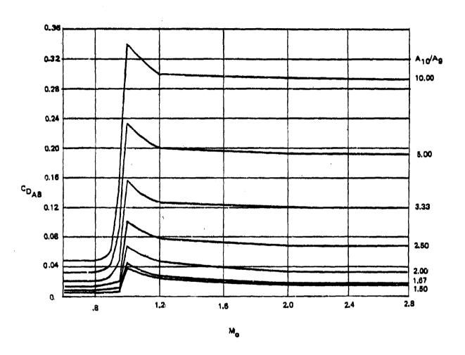
Figure 51. Drag for a Single 2-D C-D Nozzle/Aftbody Installation
