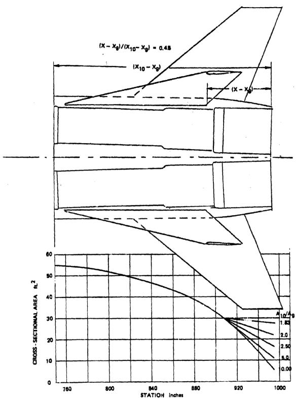
Figure 52. Nozzle/Aftbody Area Distribution for a Twin 2-D C-D Nozzle
