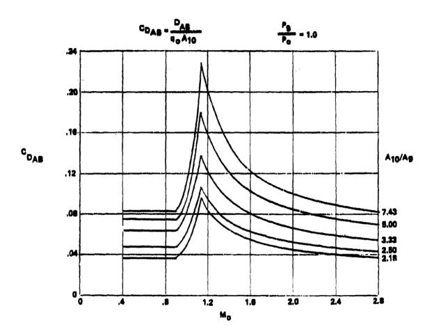
Figure 45. Drag for a Twin Round C-D Nozzle Installation
