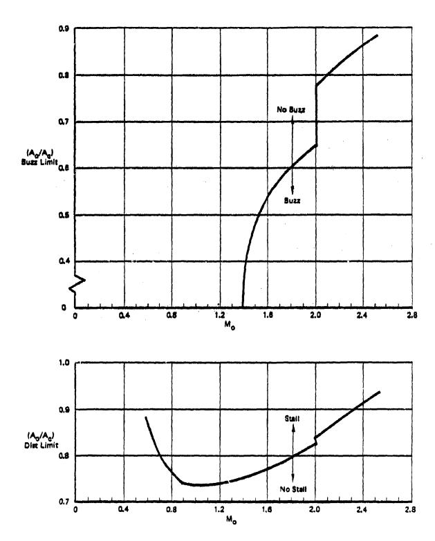
Figure 29. Performance Characteristics for Inlet Configuration #13 (continued)
