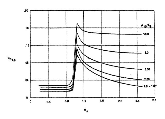
Figure 57. Drag for a Twin 2-D Wedge Nozzle Configuration
