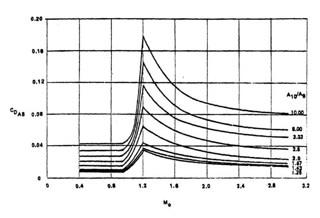
Figure 55. Drag for a Single 2-D Wedge Nozzle/Aftbody Installation
