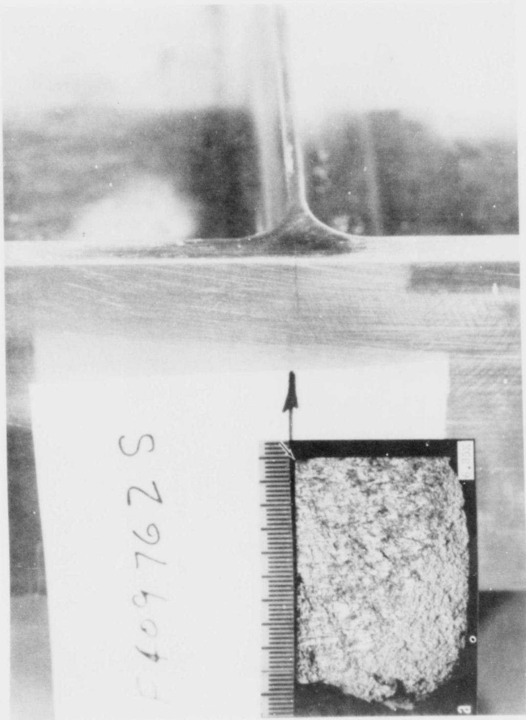
FIGURE F-6 ALUMINUM I-BEAM FAILURE, S/N F409762
