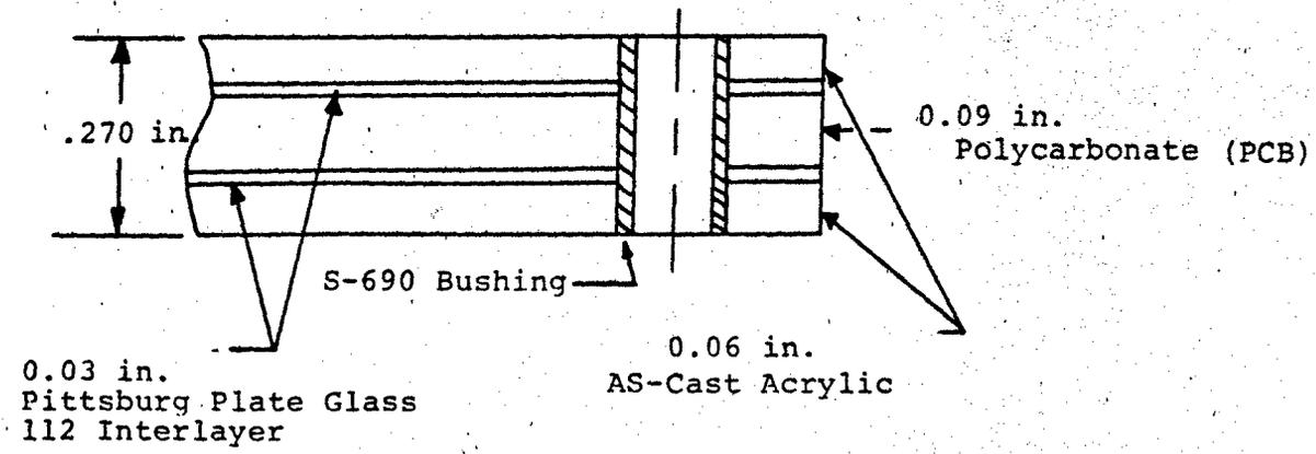
FIGURE 3. SIDE PANEL CONSTRUCTION, (Acrylic Sandwich)
