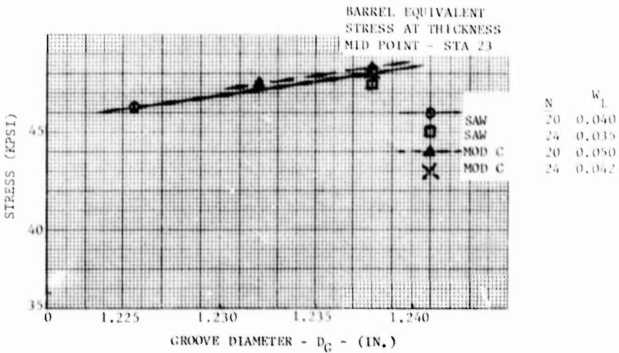
Figure 30. Barrel Stress Trends
