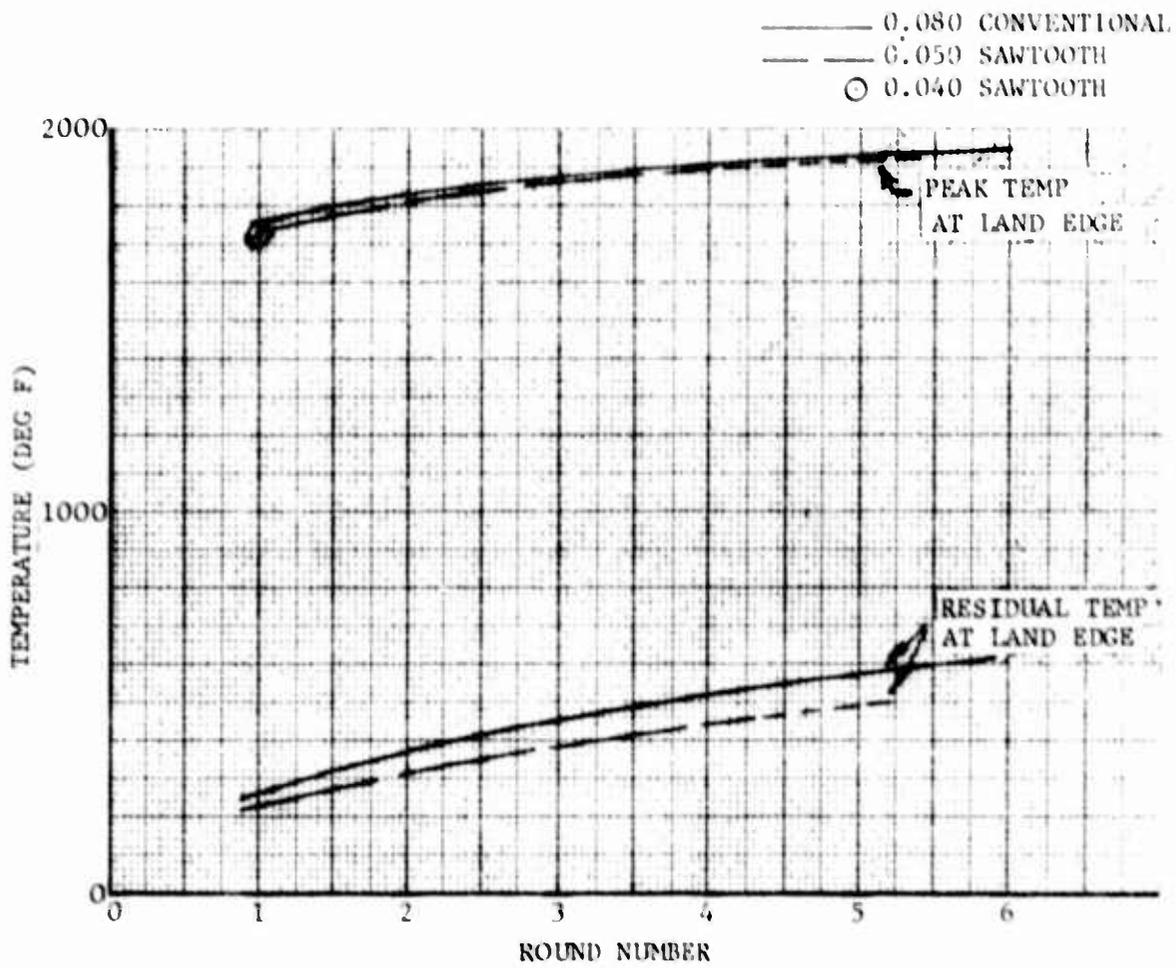
Figure 10. Comparison of Critical Land Surface Temperatures
