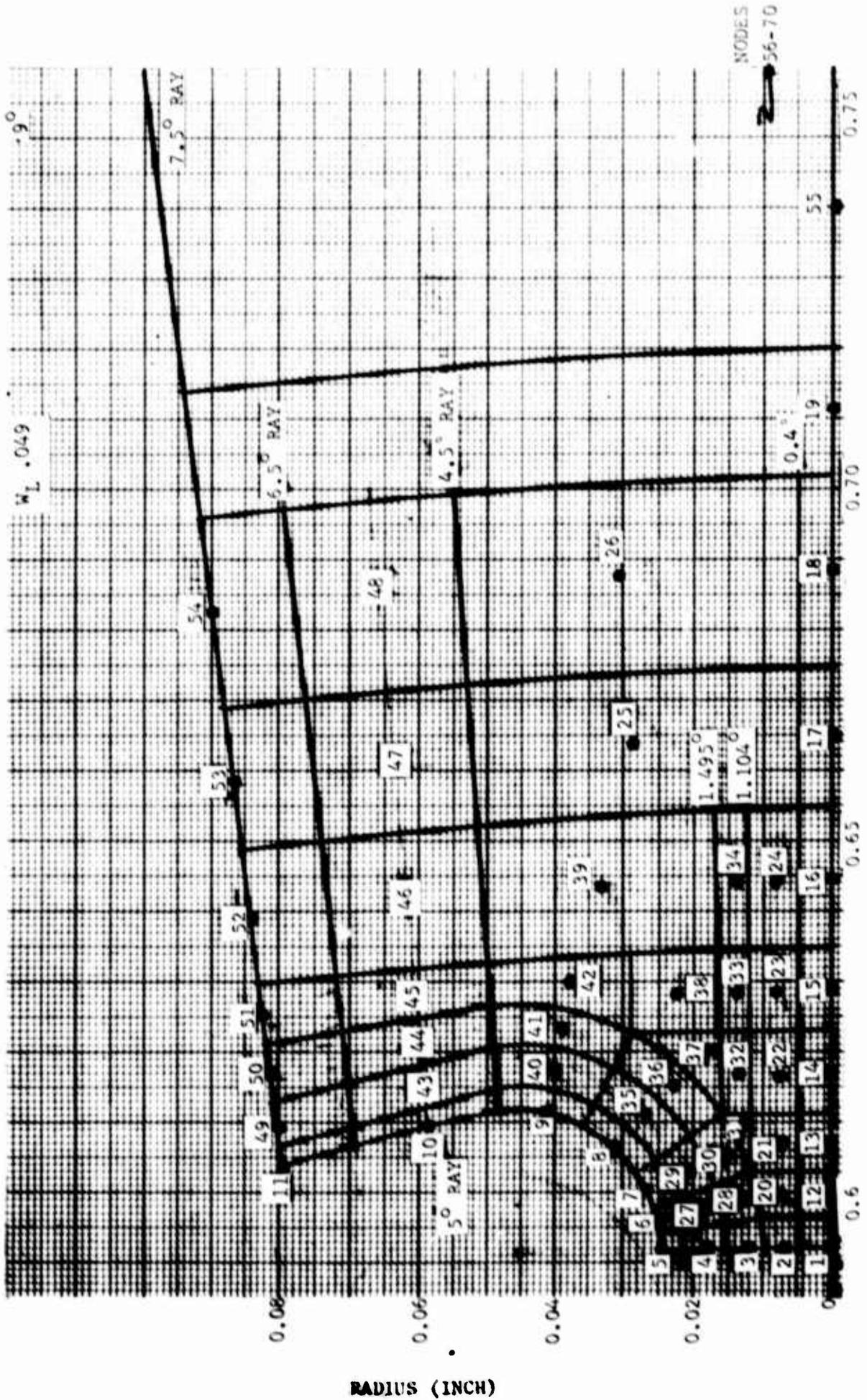
Figure 8. Two Dimensional Thermal Analysis - Nodal Matrices
