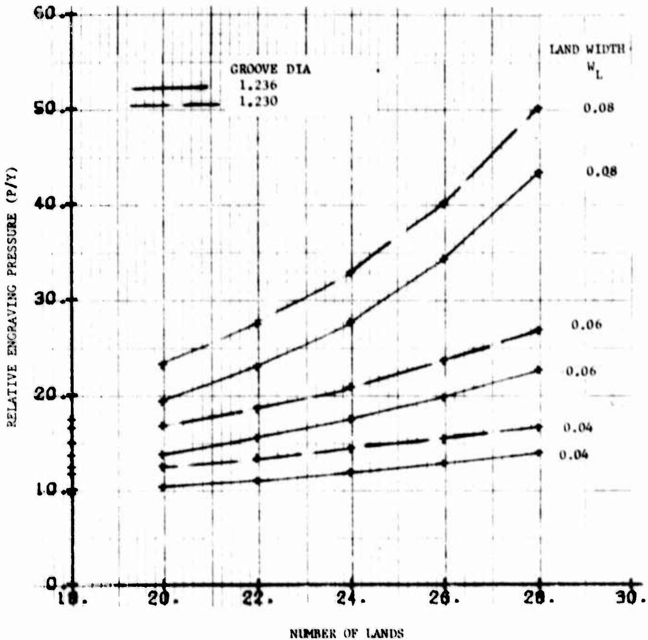
Figure 16. Relative Band Engraving Pressure Modified Conventional Rifling
