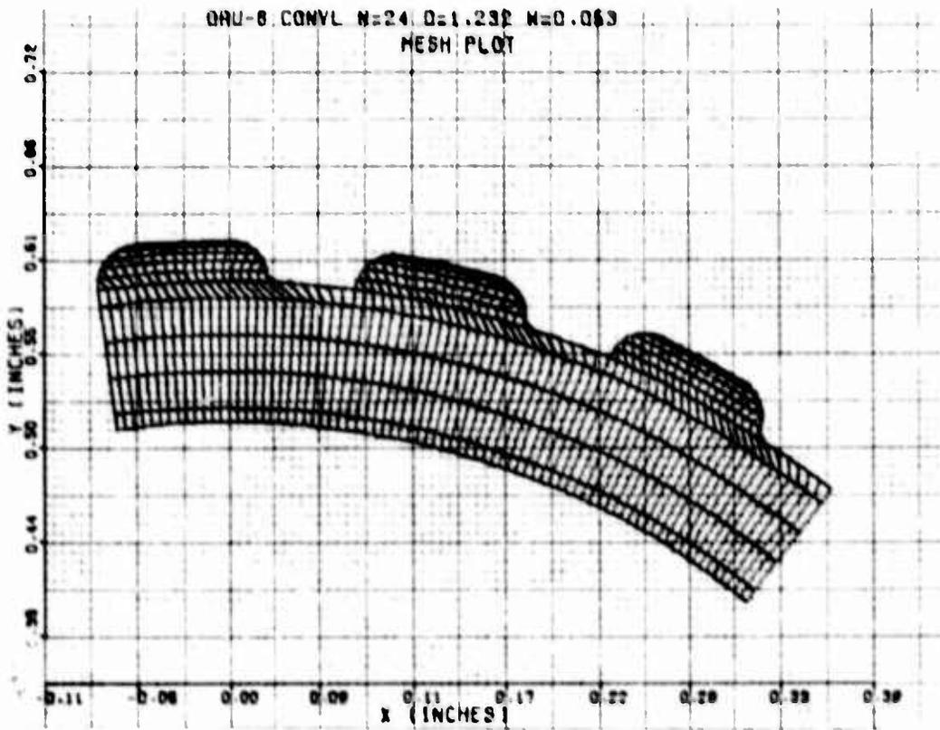
Figure 23. Typical Mesh Plot - Modified Conventional Rifling
