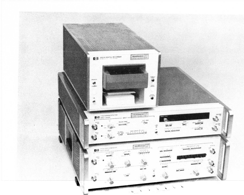
Figure 1-2 HP data generator, error detector and printer purchased for this program and delivered to ECOM.
