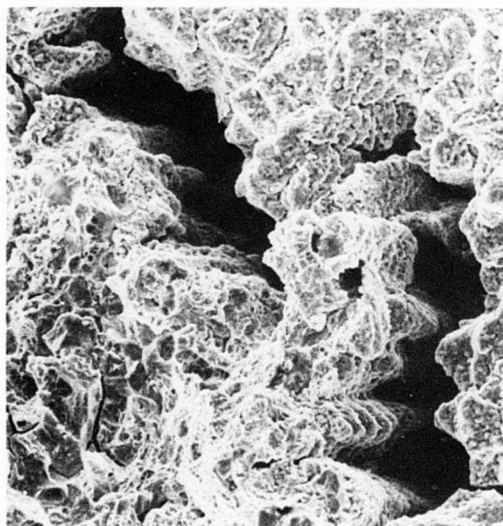
Figure V-21. FAILURE ORIGINS OF STRESS CORROSION SPECIMEN (STEELS, INTERGRANULAR CRACKING)
