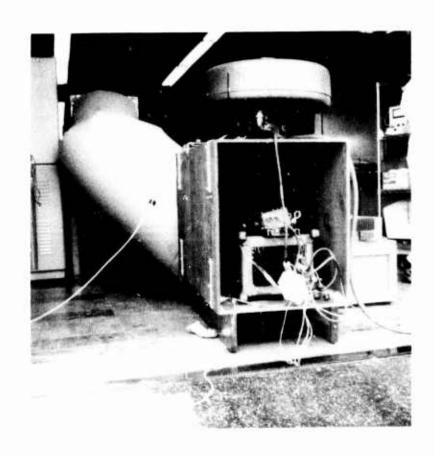
RAIN TEST SET-UP FOR RT-1202/T
